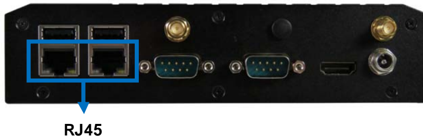
Figure 5 RJ45 connector
