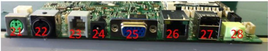
Figure 17. HK870E Connectors
