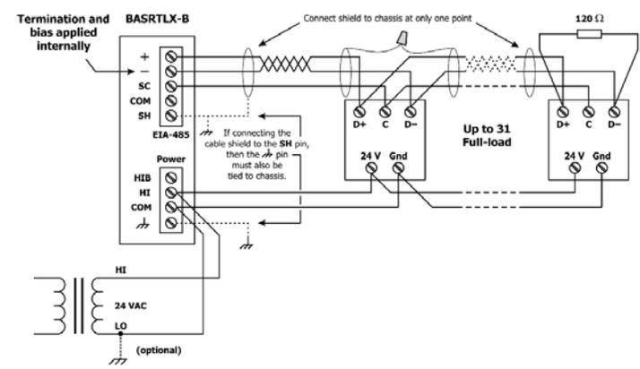
For MS/TP devices that use a power source separate from the BASRTLX-B
