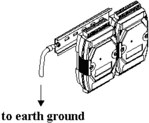
The diagram shows two DRS-125 modules mounted on a DIN rail. A wire is connected to the rail, and an arrow points to it with the text "to earth ground".
