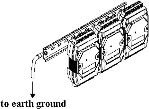
The diagram shows three DRS-240 modules mounted on a DIN rail. A wire is connected to the rail, and an arrow points to it with the text "to earth ground".
