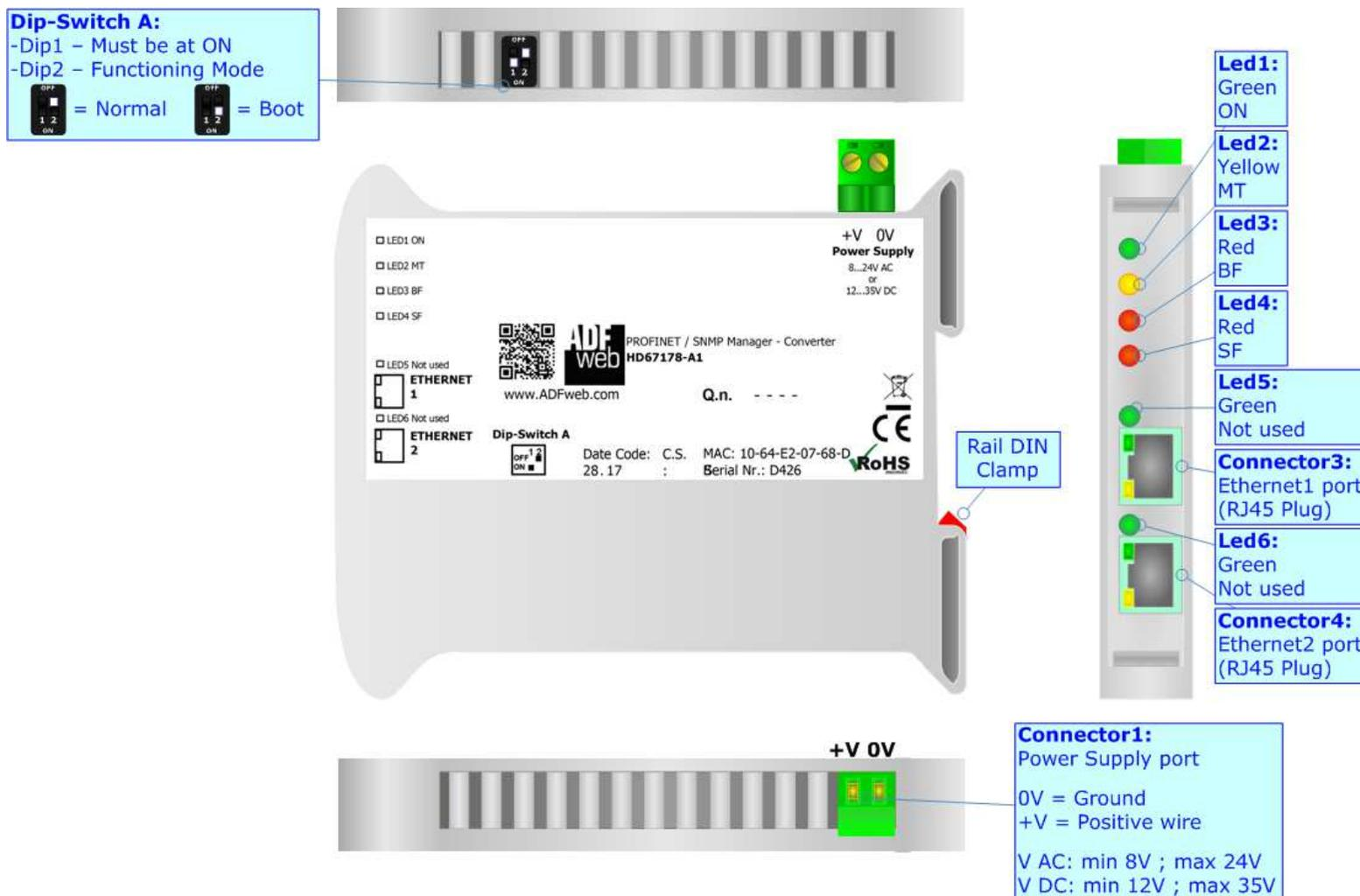
Figure 1: Connection scheme for HD67178-A1
