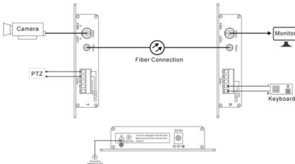
To install, connect the video inputs to the SWV60101-T, connect the video monitors or other video receptors to the SWV60101-R, and connect an appropriate optical fiber between the SWV60101-T and SWV60101-R optical ports. Connect data signal sources or destinations, as required, to the "DATA" port per the following Built-In Data Connection section.
