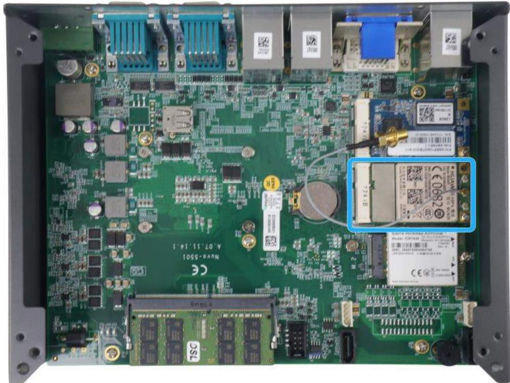
1. Please refer to the section "[Disassembling the System](#)", you may not need to completely dismantle the system to gain access to the mini-PCle slot.
