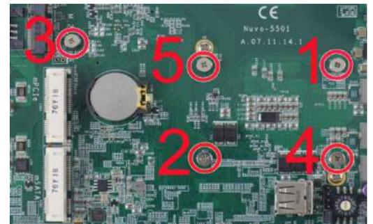
**Secure five CPU/ heatsink spring screws in order**
