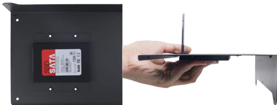
4. Connect 2.5" HDD/ SSD to the system with SATA cable.
