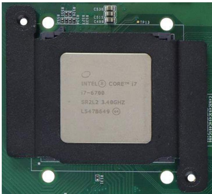
6. Turn the motherboard around and secure the bracket by tightening two M3 P-head screws.
