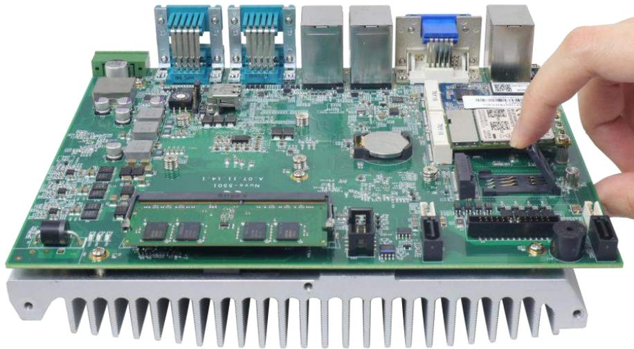
3. Shut the SIM holder and secure it by sliding the holder towards the center of the motherboard.
