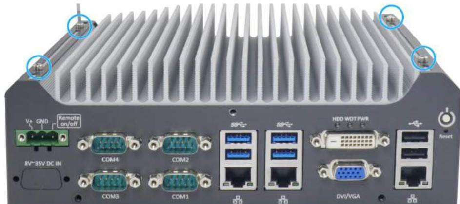
3. Unscrew the three (3) screws (indicated in blue) to remove the rear panel.
