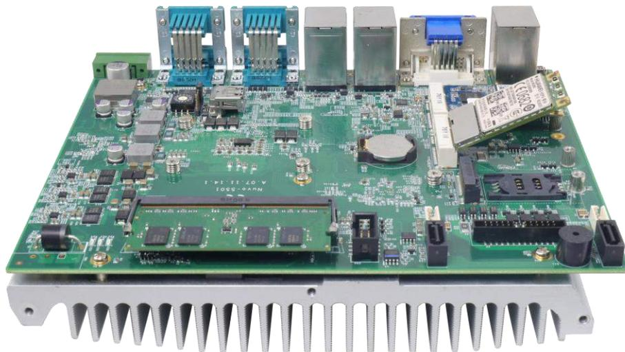
3. Gently press down and secure the module with two M2.5 P-head screws
