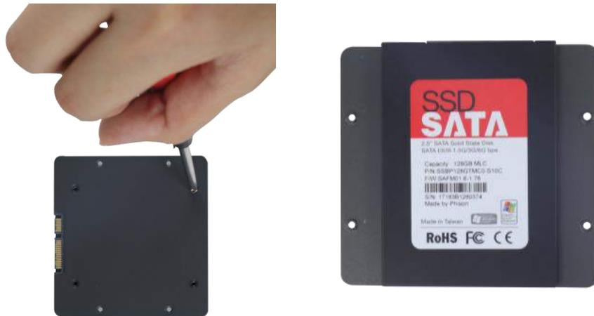
3. Secure 2.5” HDD/ SSD and the bracket on the chassis with #6-32 flat head screw.
