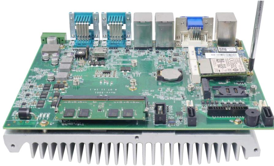
4. Clip on the IPEZ-to-SMA cable to the module and secure the antenna to the side panel. Please refer to the module's manual for clip-on connection.
