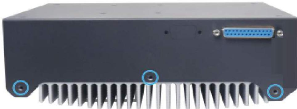
4. Unscrew the four (4) screws at the bottom of the system holding the four rubber stands.
