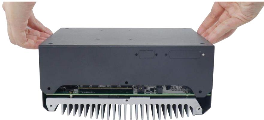
6. For Nuvo-5501-DIO, you must disconnect the DIO connection cable to the motherboard before you can remove the enclosure completely.
