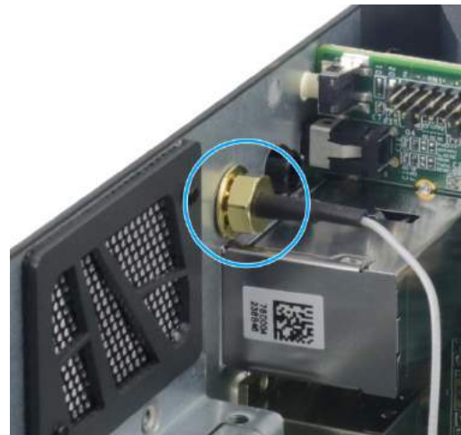
Secure antenna to rear panel
