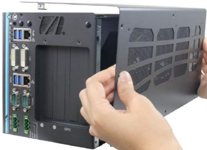
Place side panel onto enclosure
