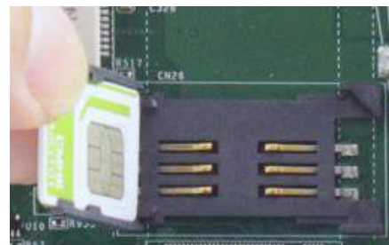
Insert SIM card with pins facing up
