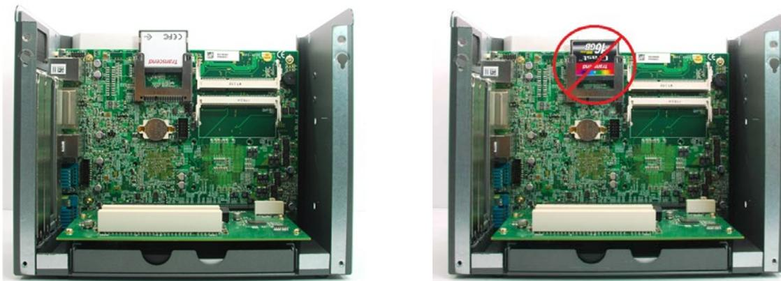
3. Push down your CFast card until it's firmly contacted with pins of the CFast socket.
