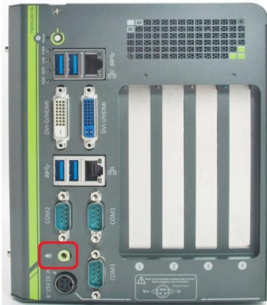
Nuvo-4000 provides audio function using Intel® High Definition Audio (built-in in HM76) and Realtek ALC262 codec. There is an audio jack available on the front panel for speaker output. To utilize the audio function in Windows, you need to install corresponding drivers for both Intel® HM76 PCH and Realtek ALC262 codec. Please refer to section 4.3 for information regarding driver installation.
