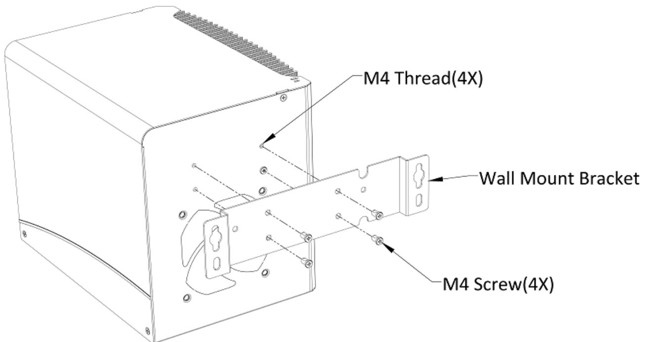
2. Fix Nuvo-4000 on the wall via the screw holes of the mounting bracket. You can also take advantage of the keyhole-shaped holes of the mounting bracket to suspend Nuvo-4000 on the Wall.
