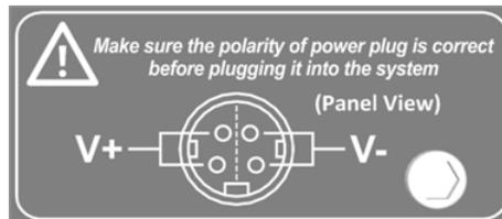
To connect DC power via the 4-pin mini-DIN power connector, please follow the steps listed below.
