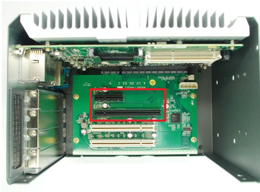
Nuvo-4022 provides one x4 and one x16 PCI Express slot. As each PCI Express lane delivers 500 MB/s bandwidth, its x4 PCI Express slot delivers 2 GB/s bandwidth and x16 slot delivers 4 GB/s bandwidth\*. In addition, a dedicated 48W (4A@12V) power rail is supplied to the x16 PCI Express slot for powering a high-watt PCIe card (e.g. a graphics card). Another 48W (4A@12V) power rail is shared by x4 PCIe Express slot and other peripheral devices.
