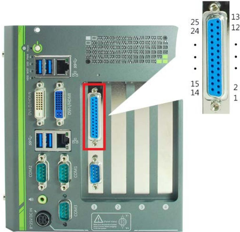
DIO Connector (DSub-25) on the front panel
