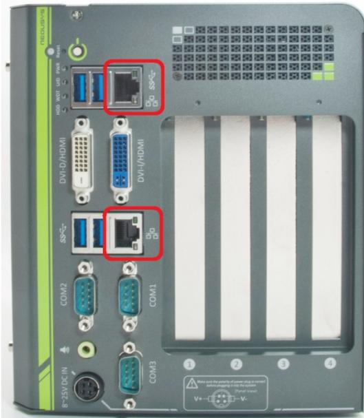
Nuvo-4000 offers two Gigabit Ethernet ports using Intel® I210 GbE controller. Each port has one dedicated GbE controller and one dedicated PCI Express link to present maximal network performance. When plugging in the Ethernet cable, you can tell the Ethernet status and speed from the LED indicators on the RJ45 connector as following:
