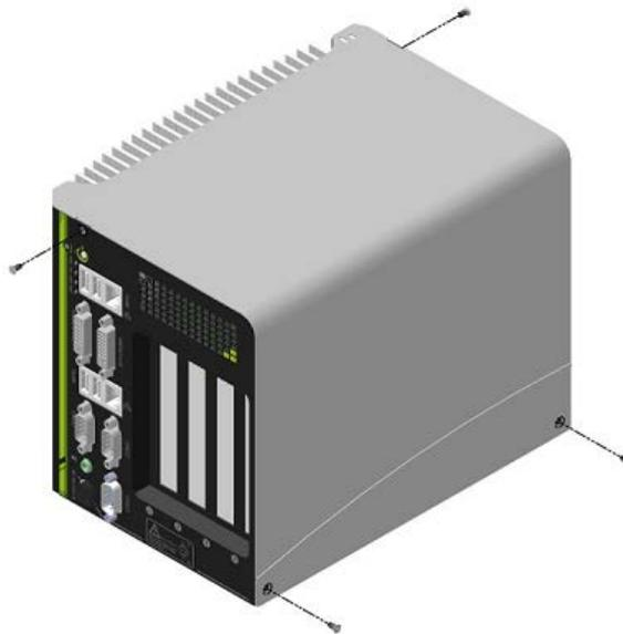
2. Simply open the chassis by pushing its side cover toward top, then remove the side cover and the SBC is exposed.
