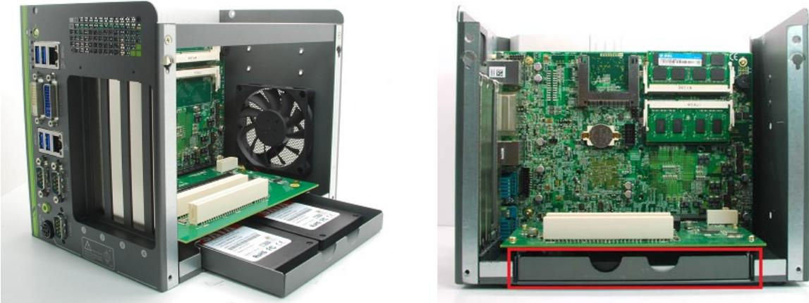
6. Fix the SATA HDD bracket to the bottom of chassis with three M3 flat-head screws.
