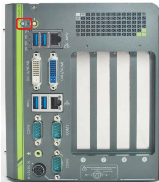
The reset button is used to manually reset the system in case of any abnormal condition. To avoid unexpected operation, the reset button is hidden behind the front panel. You need to use a pin-like object to push the reset button.
