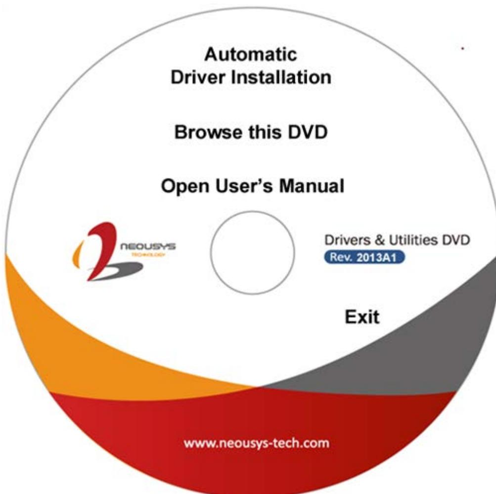
1. Click on the “**Automatic Driver Installation**”. The setup utility will automatically detect your Windows operating system and install all necessary drivers. According to different versions of Windows, the installation process takes about 6~8 minutes. Once driver installation is done, the setup utility reboots your Windows and your system works normally afterward.
