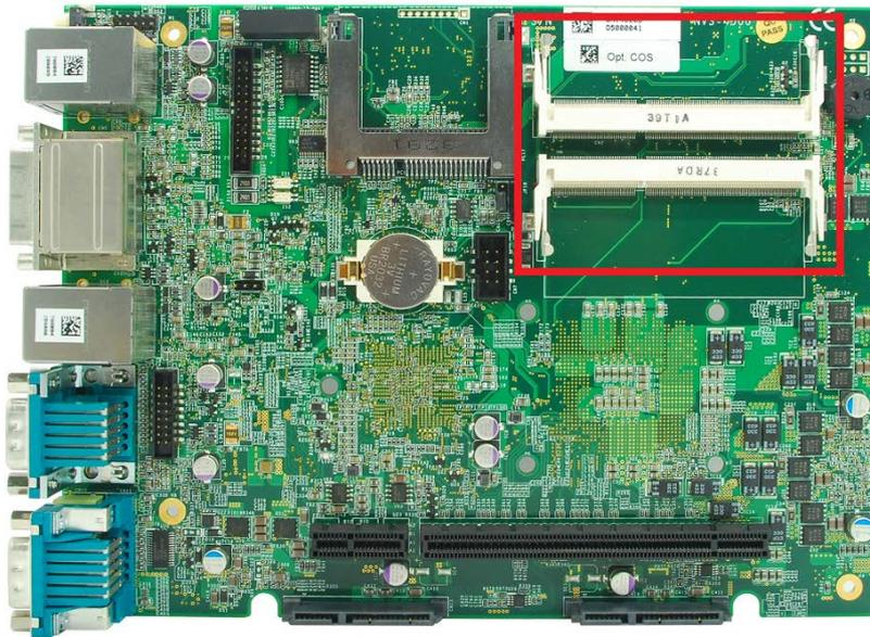
Nuvo-4000 provides two 204-pin, SODIMM sockets for installing DDR3 memory modules. It supports a maximal 16GB capacity by installing two 8GB DDR3 1600MHz SODIMM modules. For information of installing DDR3 memory modules, please refer to section 3.3 for detail.
