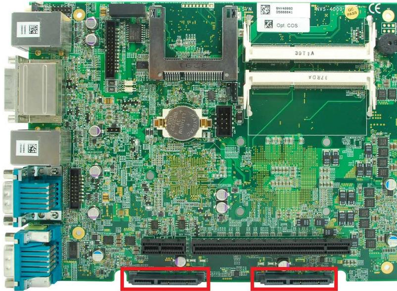
Nuvo-4000 provides two SATA ports to accommodate two 2.5" SATA hard drives in its chassis. These SATA ports are located on the SBC via two 22-pin SATA connectors. With the HDD bracket shipped with Nuvo-4000, you can directly mount two 2.5" HDDs/SSDs to these ports. For information of installing HDD/SSD to the SATA port, please refer to section 3.1 for detail.
