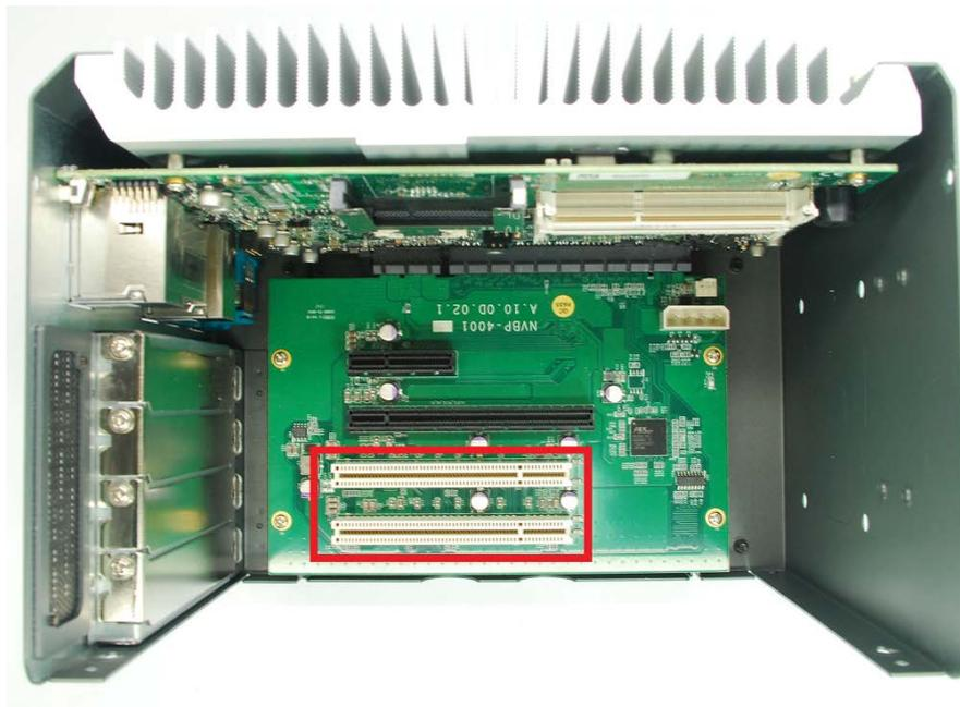
PCI slots are located on the backplane of Nuvo-4000. Nuvo-4022 provides two PCI slots, and Nuvo-4040 provides four PCI slots. These PCI slots support 5V, 32-bit/33MHz PCI bus and can accommodate the PCI card with a maximal dimension of 205mm x 105mm (PCB size, excluding connector). For information of installing PCI cards, please refer to section 3.4 for detail.
