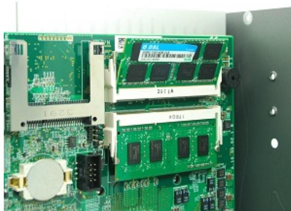
3. As the DDR3 SODIMM module is firmly contacted with socket connectors, press it down until the clamps of the socket snap into the latching position of SODIMM module.
