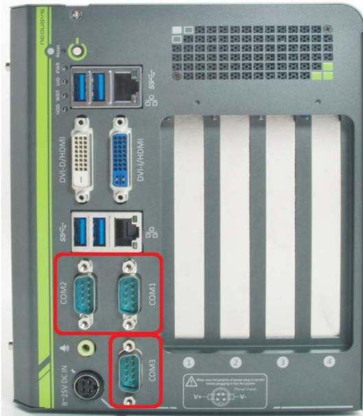
Nuvo-4000 provides three COM ports for communicating with external devices. These COM ports are implemented using industrial-grade ITE8783 Super IO chip (-40 to 85°C) and provide up to 115200 bps baud rate.
