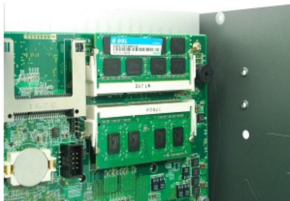
4. Repeat step#2 and step#3 if you want install second DDR3 SODIMM module.
