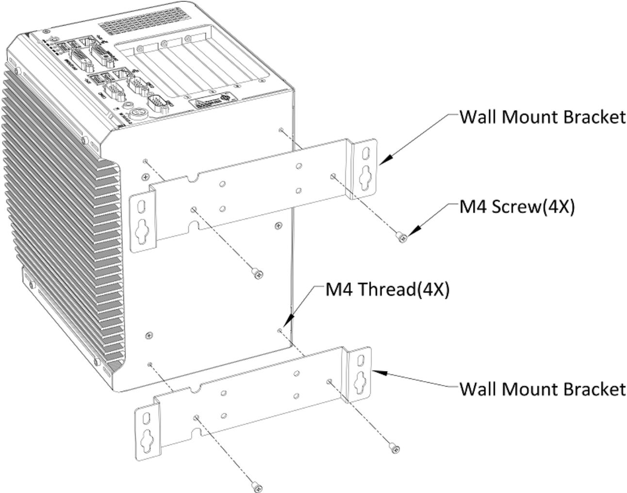
2. Fix Nuvo-4000 on a flat surface via the screw holes of two mounting brackets.
