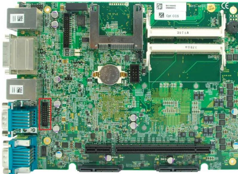
Nuvo-4000 provides additional two USB 2.0 ports internally via a 2x8 pins, 2.0mm pitch box header. The internal USB ports are designed to allow users attaching a protection dongle inside the chassis. To use the internal USB port, you need a dedicated box-header to USB cable. Please contact Neosys for further information
