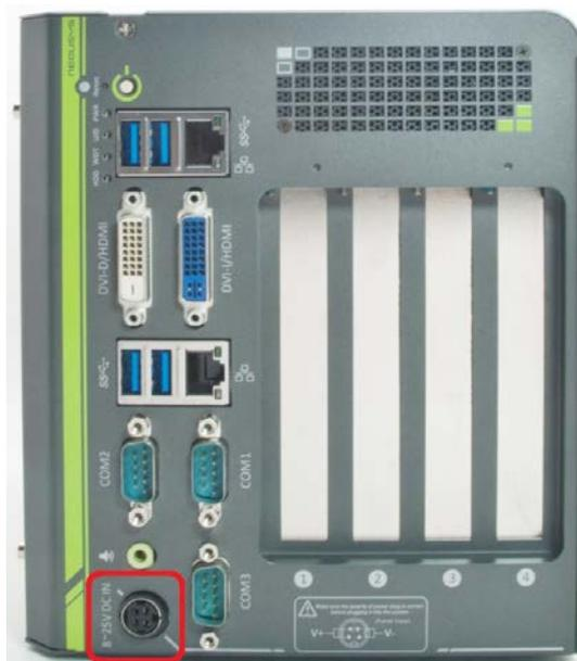
Nuvo-4000 allows a wide range of DC power input from 8 to 25V. The 4-pin mini-DIN power connector on the front panel is used to connect the power plug of an AC/DC adapter. It's convenient for indoor usage where AC power is usually available. Since there is no specific rule of pin definition for this type of connector, please always confirm the polarity of the power connector in prior to plug it into Nuvo-4000 if you're not using the power adapter provided from Neusys.
