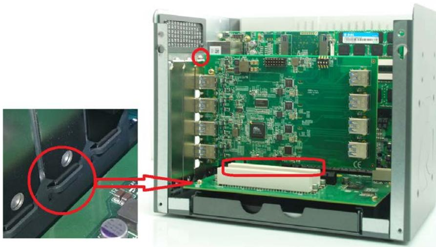
3. Get the M3 PW-head screw from the accessory box. And use it to fix your PCI/PCIe add-on card.
