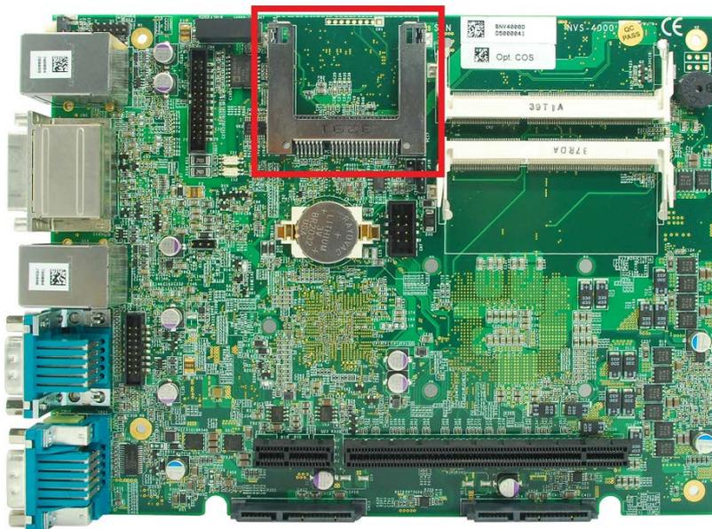
Nuvo-4000 provides a CFast socket on its SBC. CFast is a new interface for portable storage device. It shares a similar form-factor as CompactFlash but leverages Serial ATA interface to offer higher data transfer rate. The CFast socket on Nuvo-4000 is a push-push type. You can insert and push a CFast card to the end to install it, and push the installed CFast card again to eject it.
