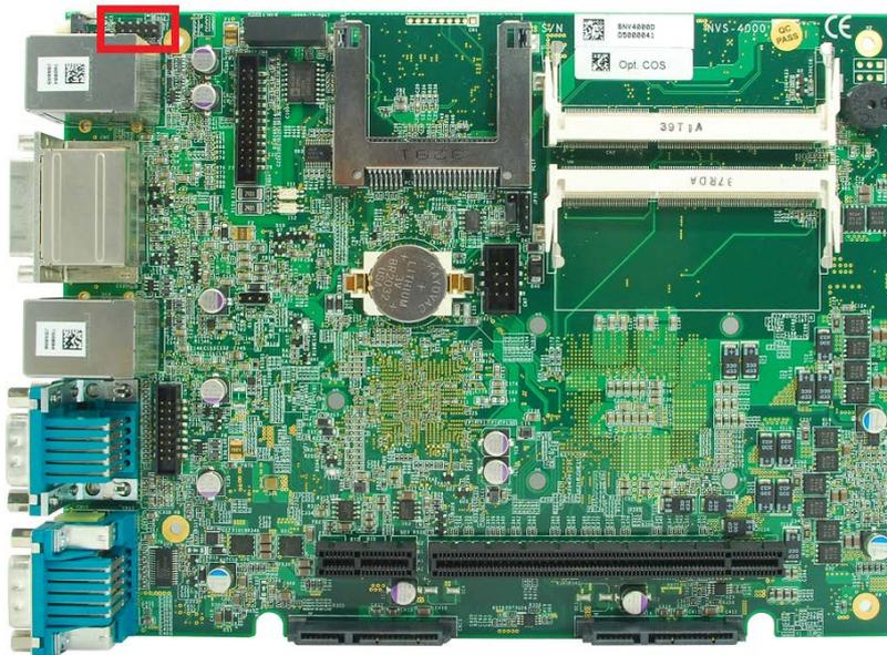
For an application which places Nuvo-4000 inside a cabinet, it's useful to output the system status to external LED indicators so that users can check how the system's running. Nuvo-4000 provides a 2x6, 2.0mm pitch pin header to output system status such as power, HDD, watchdog timer, and control system on/off remotely.
