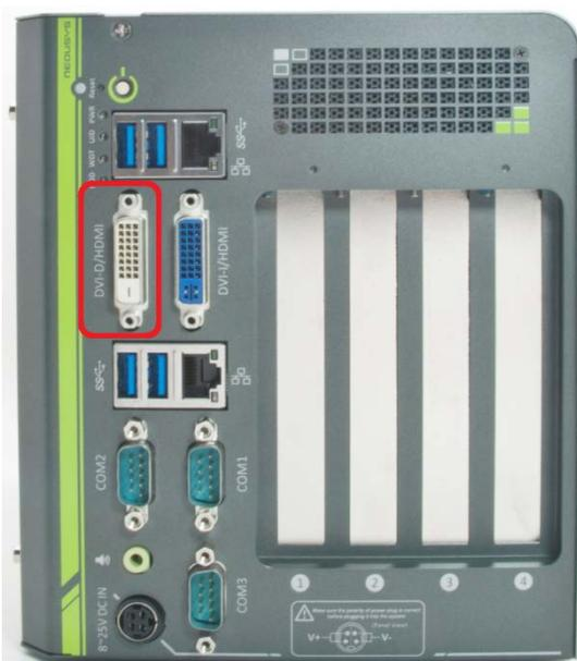
Nuvo-4000 supports triple independent display outputs via a DVI-I and a DVI-D connector. The DVI-D connector on the front panel offers DVI/HDMI signal output and supports up to 1920 x 1080 resolution. You shall need a DVI to HDMI cable when connecting to a HDMI display device.
