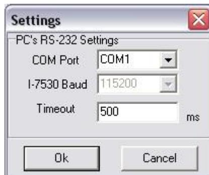
7. Press the "OK" button. Then the I-7530 Utility will show the test tab in the window as can be seen in the below figure.
