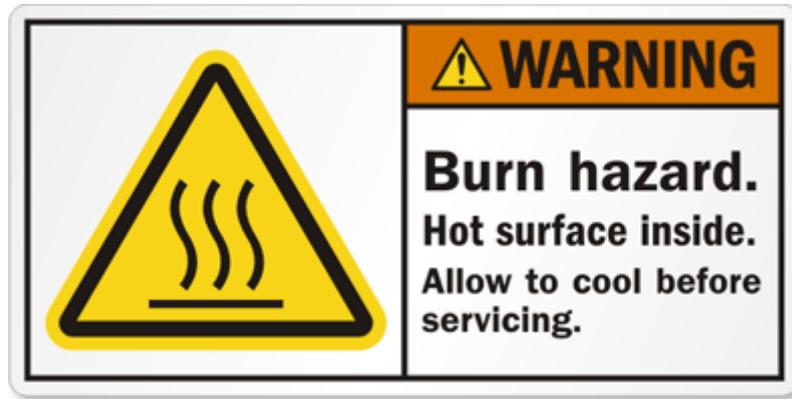
**CAUTION:** The surface temperature for the metallic enclosure can be very high! Especially after operating for a long time, installed at a close cabinet without air conditioning support, or in a high ambient temperature space. **DO NOT touch the hot surface with your fingers while servicing!!**
