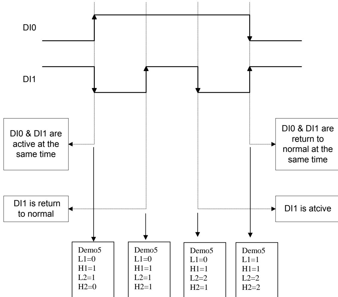
Refer to [DEMO5.C](#) for source program. All these three falling-edge and rising-edge can be detected by [DEMO5.C](#).
