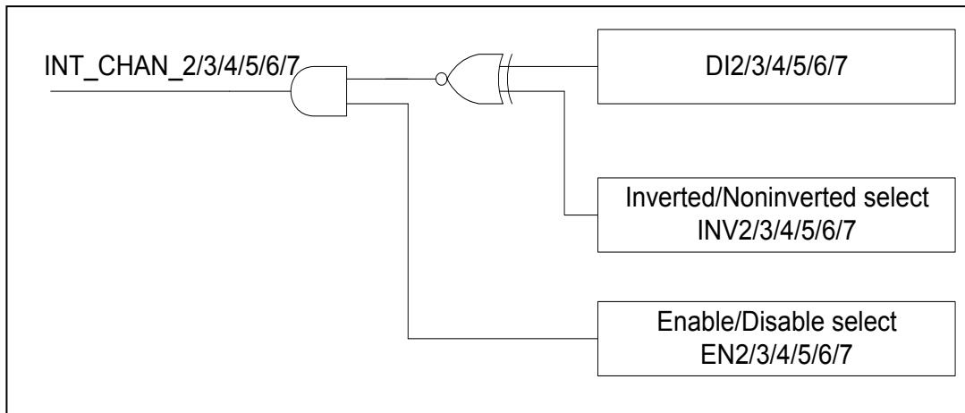
The INT\_CHAN\_2/3/4/5/6/7 must be fixed in low level state normally and generated a high\_pulse to interrupt the PC.
