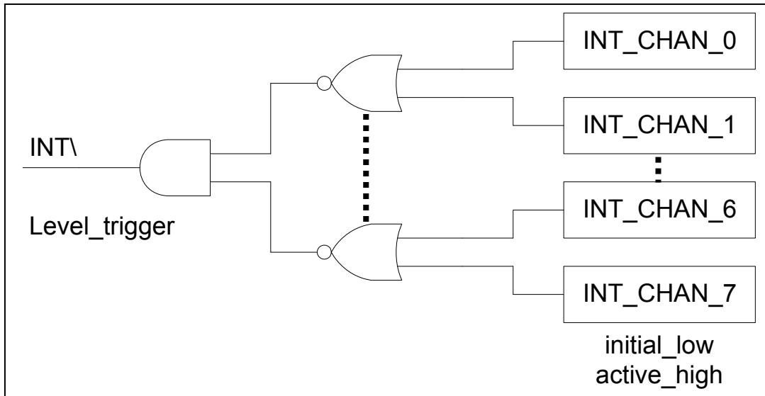
The interrupt output signal of PISO-725, INT\, is **level-trigger & Active\_Low**. If the INT\ generate a low-pulse, the PISO-725 will interrupt the PC once a time. If the INT\ is fixed in low level, the PISO-725 will interrupt the PC continuously. So the INT\_CHAN\_0/1/2/3/4/5/6/7 must be controlled in a **pulse\_type** signals. **They must be fixed in low level state normally and generated a high\_pulse to interrupt the PC.**
