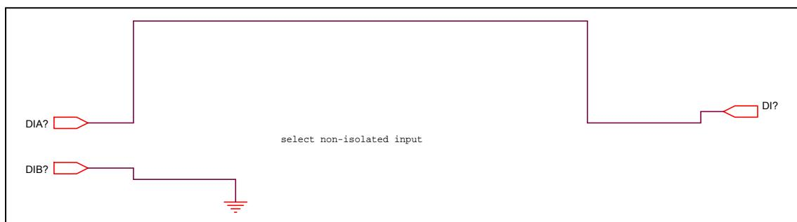
The non-isolated input is TTL compatible.
