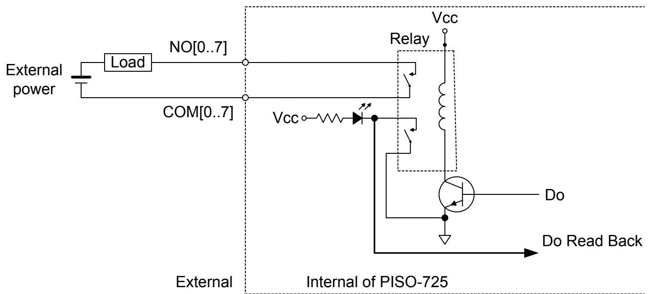
The relay of PISO-725 is 2-Form-C type as following:
