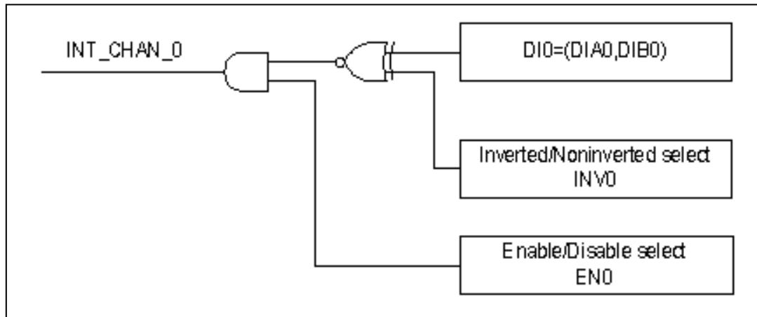
The INT\_CHAN\_0 must be fixed in low level state normally and generated a high\_pulse to interrupt the PC.
