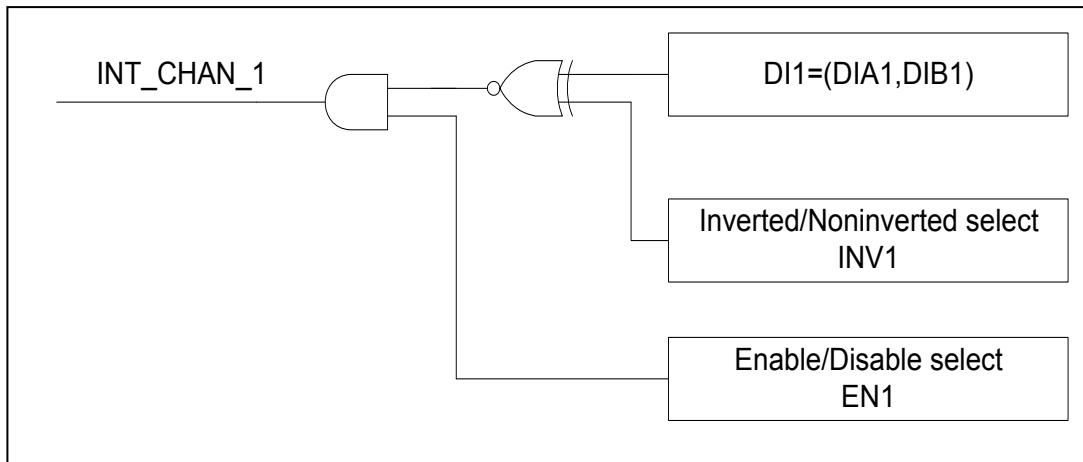
The INT\_CHAN\_1 must be fixed in low level state normally and generated a high\_pulse to interrupt the PC.
