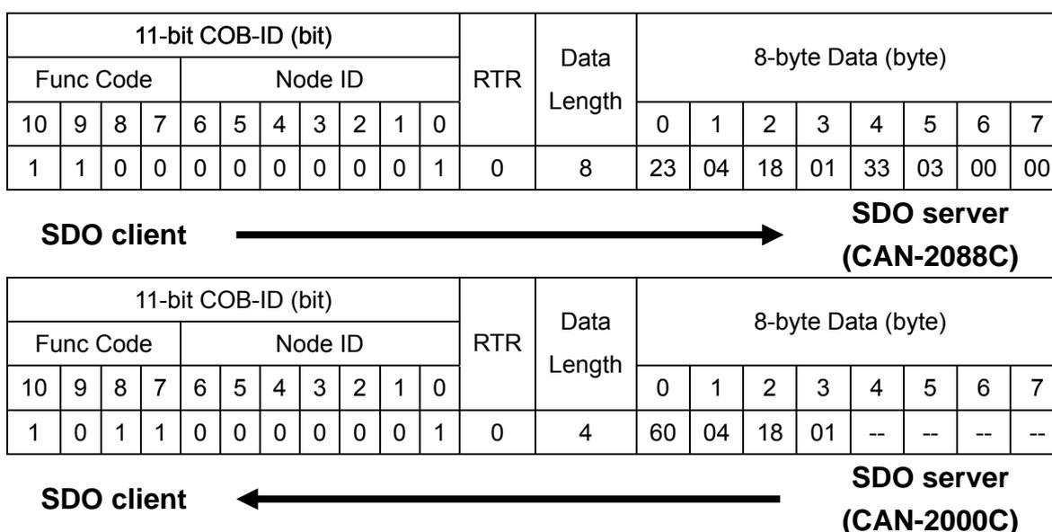
Write object index 0x1804 and subindex 1 to 0x333 means set the new COBID 0x333 to 5<sup>th</sup> TxPDO. To do this, the counter channel 6 and 7 will be mapping in the new PDO COBID 0x333. So user can use 0x333 COBID to remote the counter channel 6 and 7 data.
