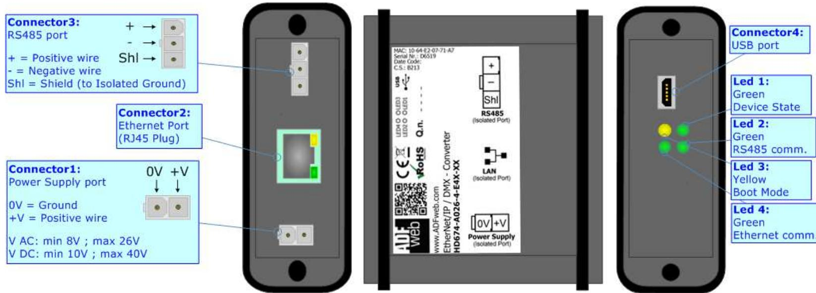
Figure 1a: Connection scheme for HD674-A026-E4x-xx
