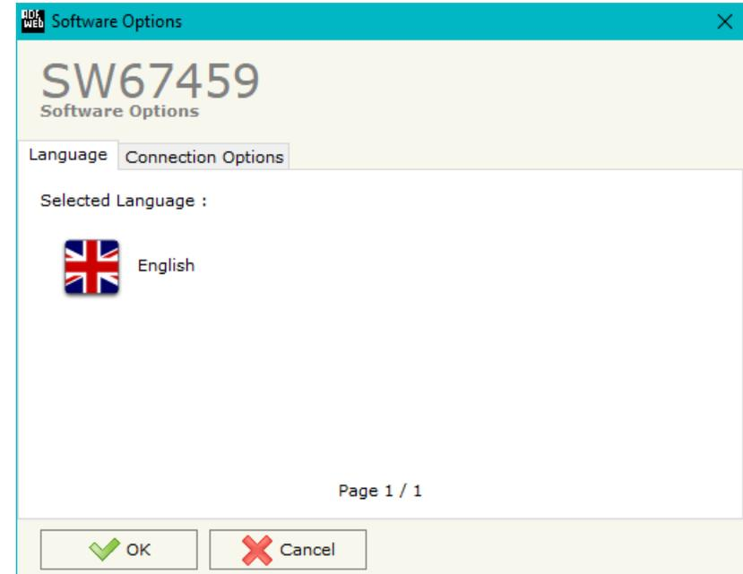
In the section “Connection Options”, it is possible to check if there are some updatings of the software compositor in ADFweb.com website. Checking the option “**Check Software Update at Start of Program**”, the SW67459 checks automatically if there are updatings when it is launched.
