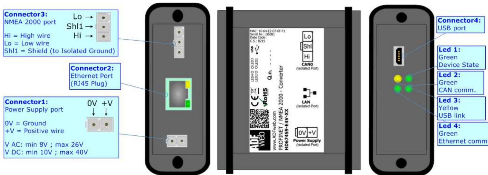
Figure 1a: Connection scheme for HD67459-E4x-xx
