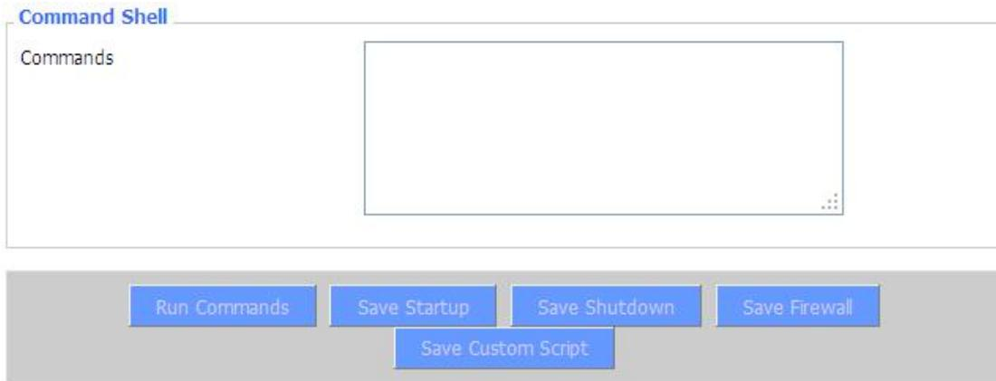
**Run Command:** You can run command lines via the web interface. Fill the text area with your command and click Run Commands to submit.
