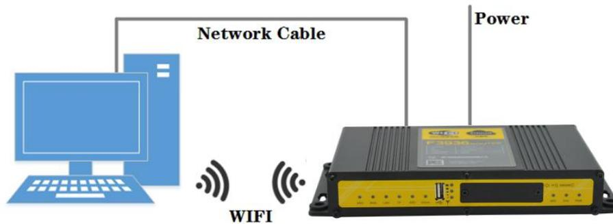
Please modify the IP address of PC as the same network segment address of the router, for instance, 192.168.1.9. Modify the mask code of PC as 255.255.255.0 and set the default gateway of PC as the router's IP address (192.168.1.1).
