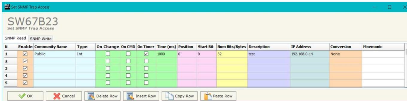
Figure 10a: **“Set SNMP Access -> SNMP Read”** window
