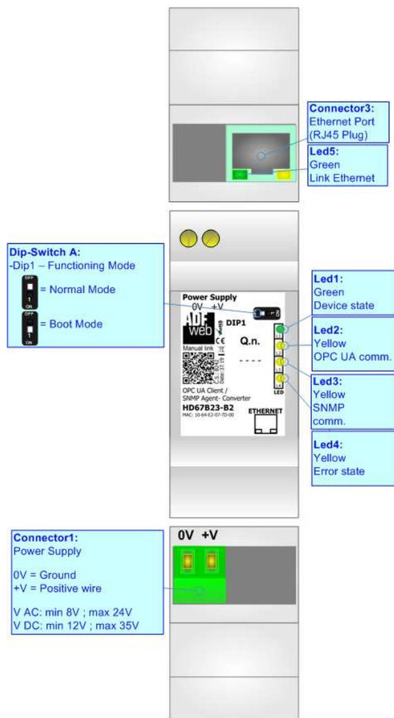
Figure 1: Connection scheme for HD67B23-B2
