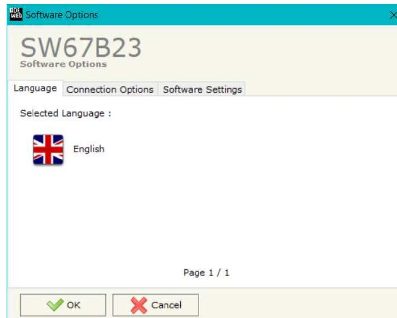
In the section “Connection Options”, it is possible to check if there are some updates of the software compositor in ADFweb.com website. Checking the option “**Check Software Update at Start of Program**”, the SW67B23 check automatically if there are updates when it is launched.
