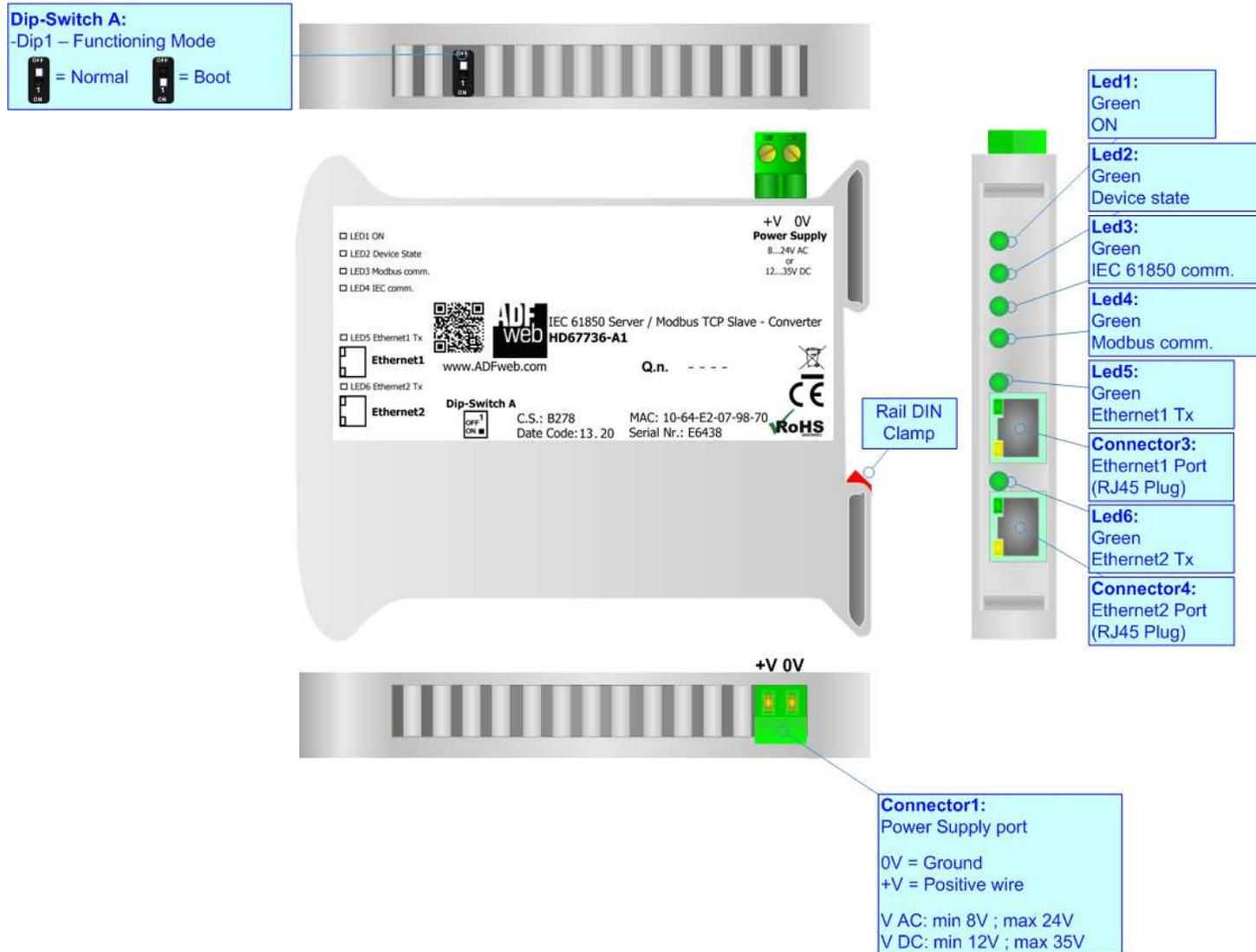
Figure 1: Connection scheme for HD67736-A1
