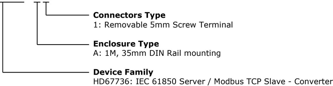
Order Code: **HD67736-A1** - IEC 61850 Server / Modbus TCP Slave - Converter
