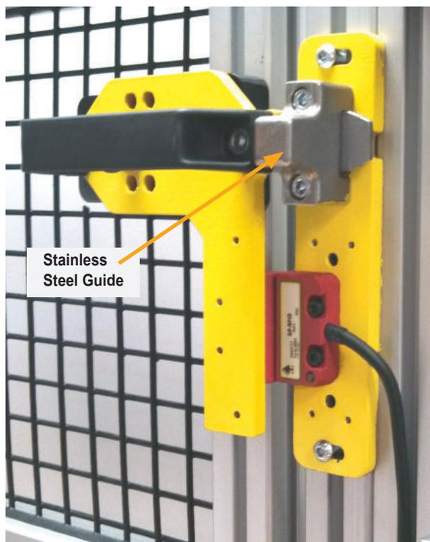
**GBN-1** shown fitted with SPF-RFID Non Contact Switch
