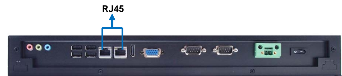
Figure 5 RJ45 connector
