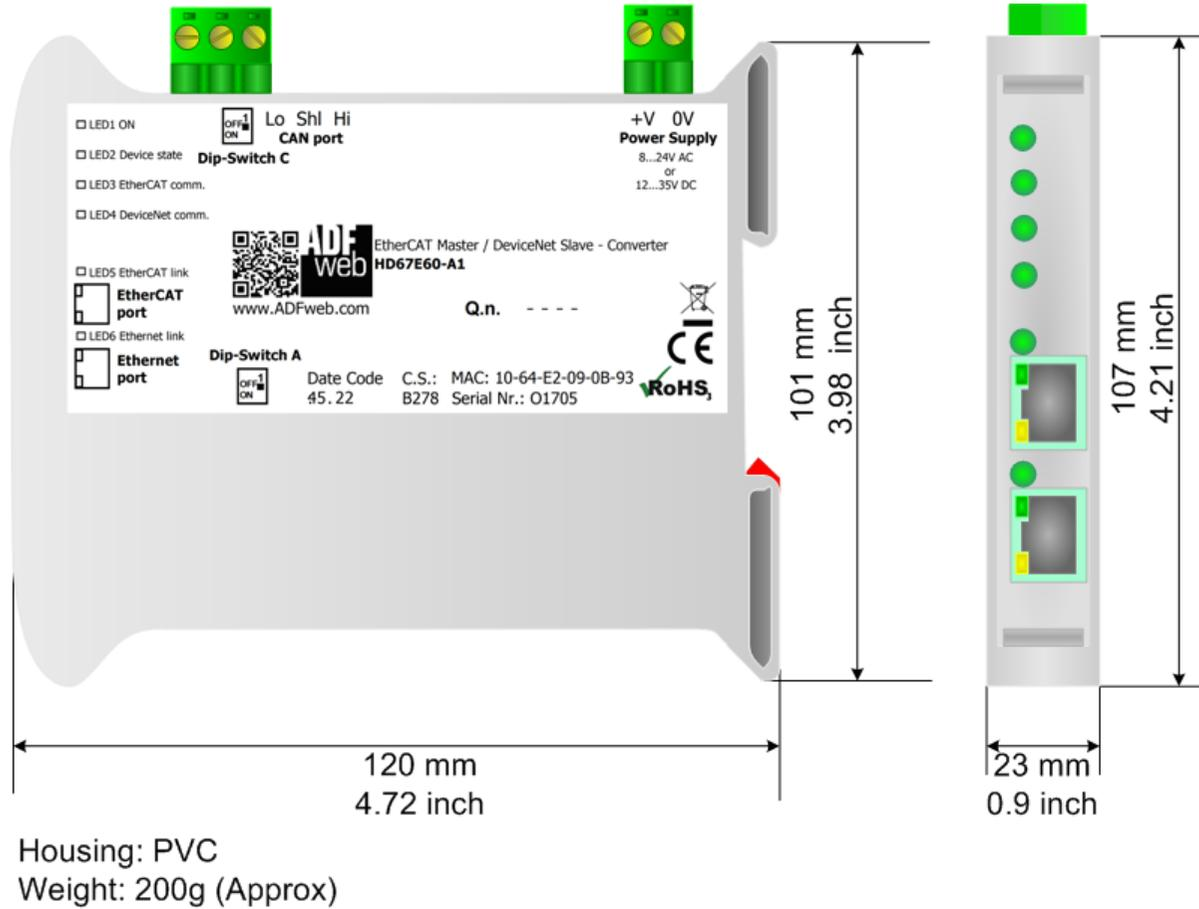
Figure 7: Mechanical dimensions scheme for HD67E60-A1
