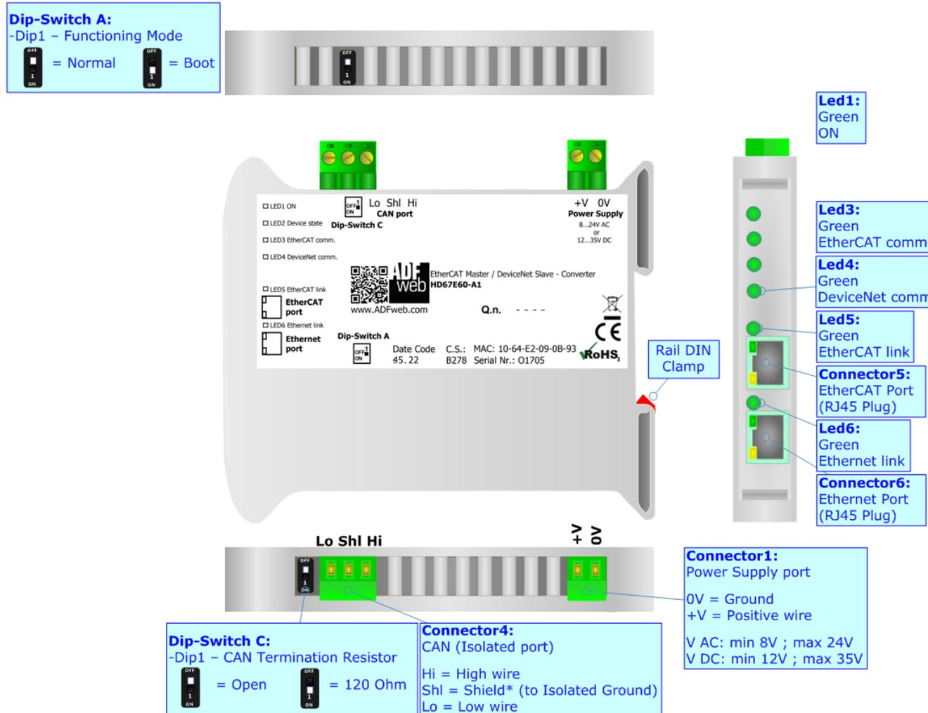
Figure 1: Connection scheme for HD67E60-A1
