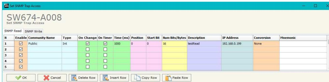
Figure 5a: **“Set SNMP Access -> SNMP Read”** window
