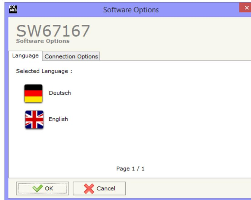
In the section “Connection Options”, it is possible to check if there are some updatings of the software compositor in ADFweb.com website. Checking the option “**Check Software Update at Start of Program**”, the SW67167 check automatically if there are updatings when it is launched.
