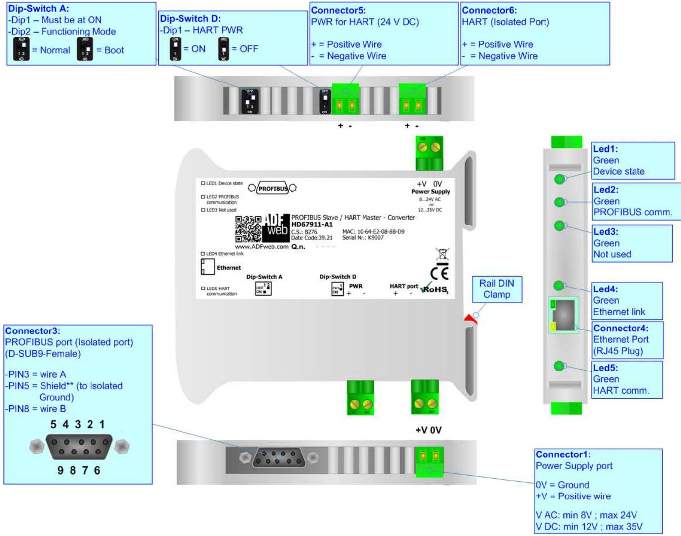
Figure 1: Connection scheme for HD67911-A1
