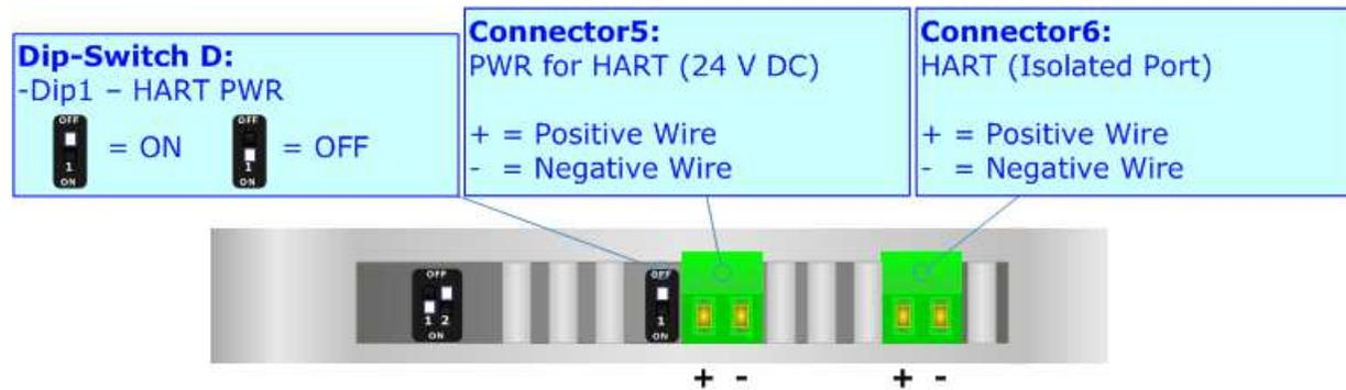
It is possible to provide the current loop for HART communication and an additional low power supply @ 24 V DC for feeding HART devices by setting Dip-Switch D at ON position. Current loop for HART is required when there is not an external device in the bus that provides it.
