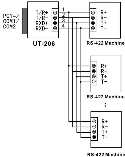
3. Half-duplex communication connections between UT-206 interfaces
