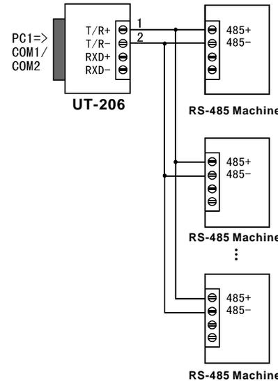
3. Half-duplex communication connections between UT-206 interfaces
