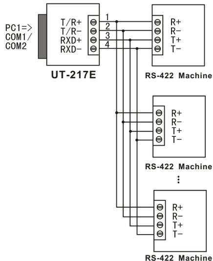
3. Half-duplex communication connections between UT-217E interfaces
