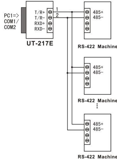
3. Half-duplex communication connections between UT-217E interfaces
