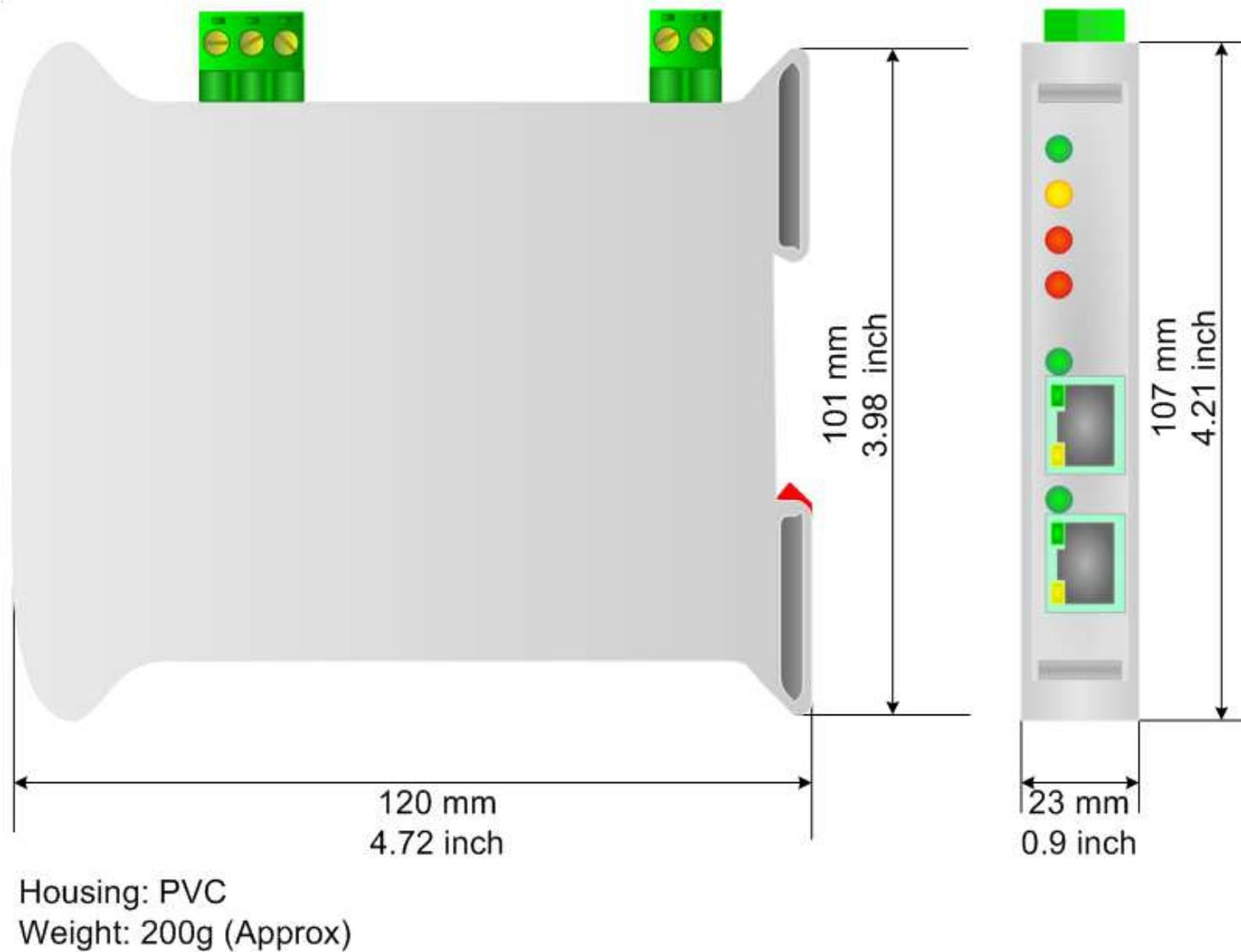
Figure 10: Mechanical dimensions scheme for HD67608-A1
