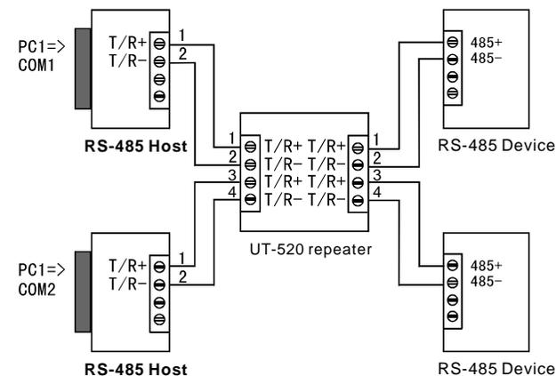
2. RS-485 point-to-multipoint / 2-line half duplex relay communication
