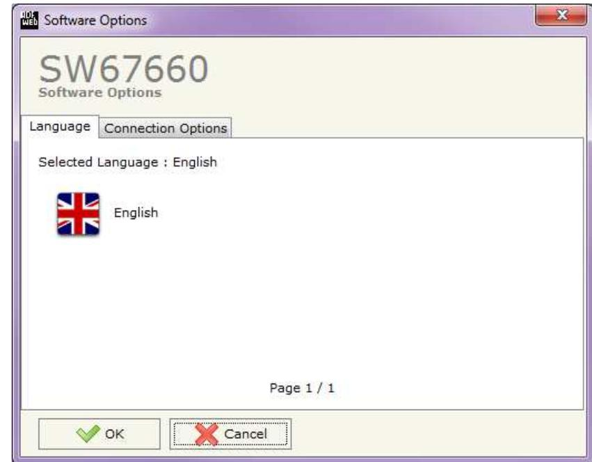
In the section “Connection Options”, it is possible to check if there are some updatings of the software compositor in ADFweb.com website. Checking the option “**Check Software Update at Start of Program**”, the SW67660 check automatically if there are updatings when it is launched.
