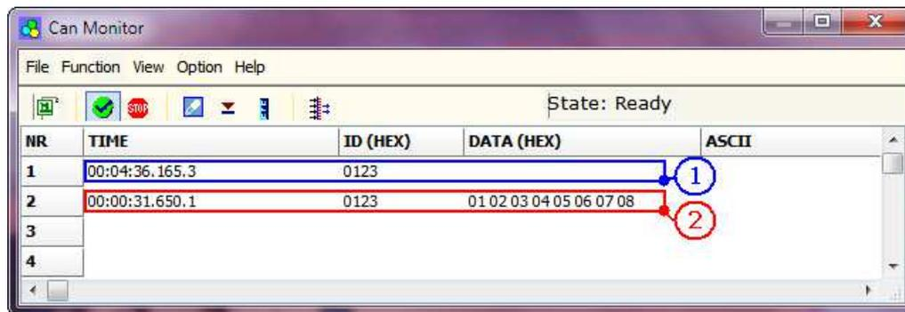
Figure 7: "Can Monitor" window for visualize the CAN frame for read request 1
