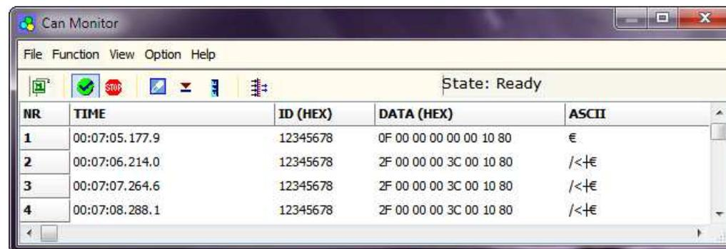
Figure 8: "Can Monitor" window for visualize the CAN frame for read request 2
