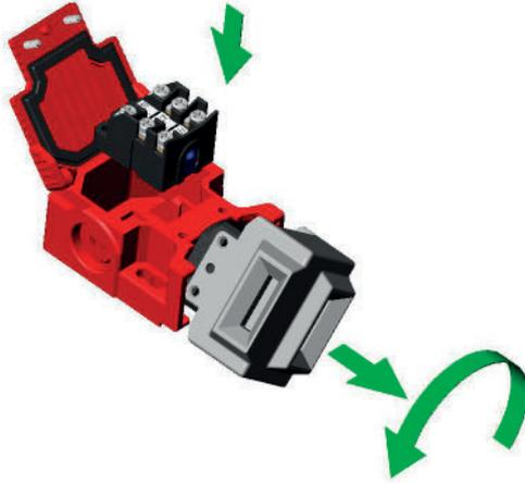
The head can be rotated to give 4 actuator entry positions. Designed with a hinged lid to fit replaceable contact blocks. Flexible actuators are available and the K-15 is available with a Stainless Steel head.
