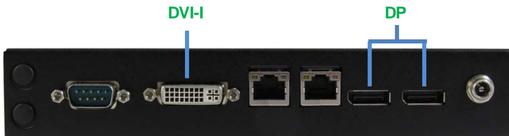
Figure 4 Connect the DVI-I / DP cable
