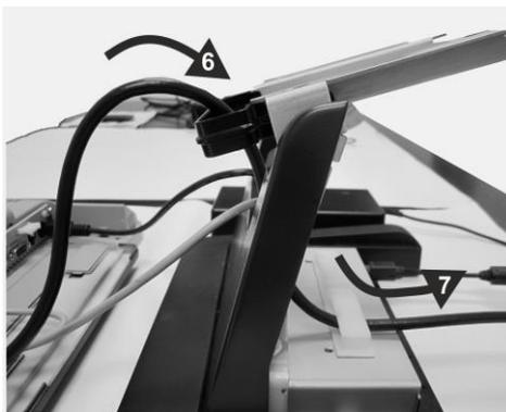
6. Pull the cable through the cable support.
