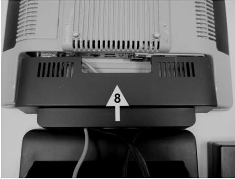
8. Place back the cable connection cover and pull the cables through the opening at the bottom.
