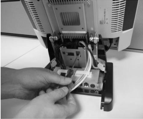
3. Secure the bracket with the screws provided.
