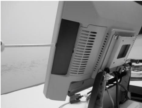
1. Remove the flap using a screw driver, exposing one end of a connecting cable.
