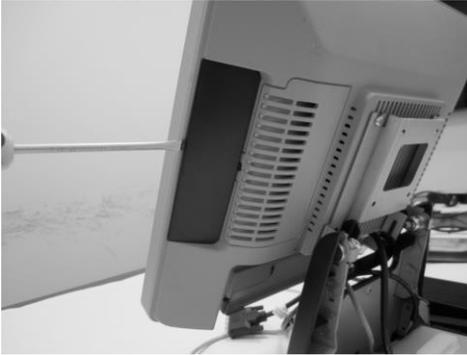
1. Remove the flap using a screw driver.
