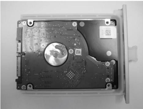
6. Replace the new hard disk and fix it back to the drive carrier.
