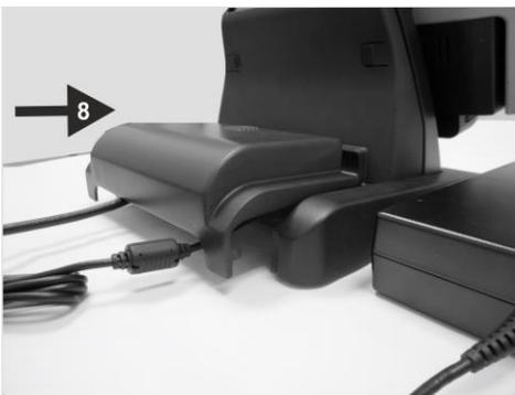
8. Place in the base cover. The installation is complete.
