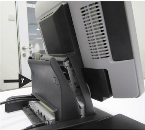
7. Place in the back cover, routing the cables through the bottom.
