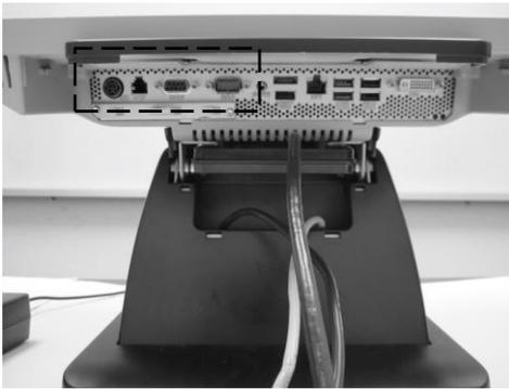
3. The HDD or SSD is in the drive carrier located on the left.
