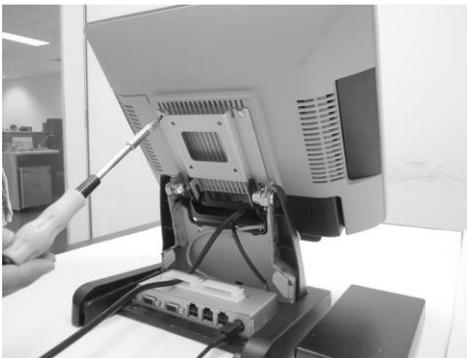
5. Tighten the four Torx screws to secure the display to the stand.
