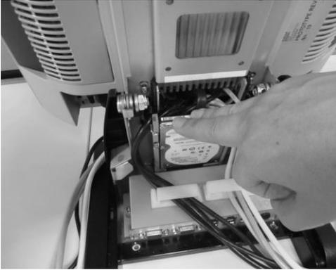
6. Apply a slight pressure to ensure that the hard disk drive assembly is engaged with the docking cables.
