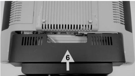
6. Place back the cable connection cover and pull the cables through the opening at the bottom.
