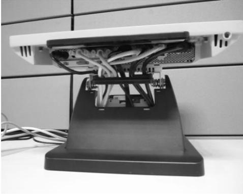
9. Connect the cables to the USB1 and eSATA connectors.
