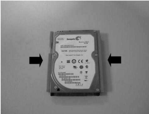
4. Assemble the guide rails to the hard disk drive.
