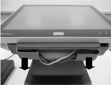
2. Pull down the cable connection cover to uncover the connector panel.
