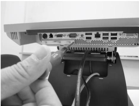
4. Remove both screws that fix the drive carrier to the connector panel and pull out the drive carrier.
