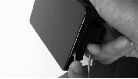
2. Release the catch on one side of the peripheral's holder.
