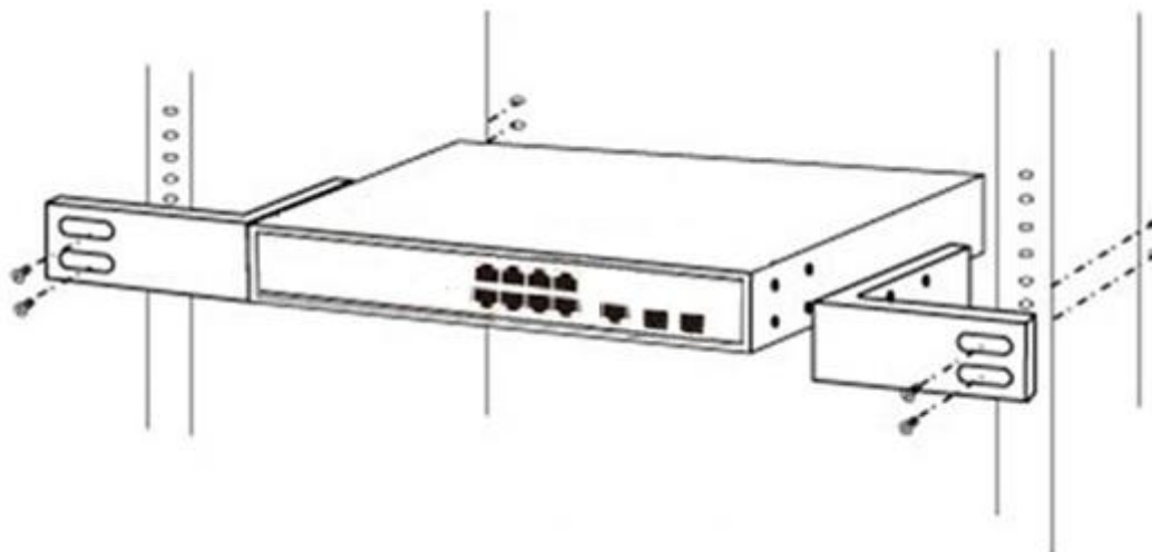
Figure 5 - Rack Installation
