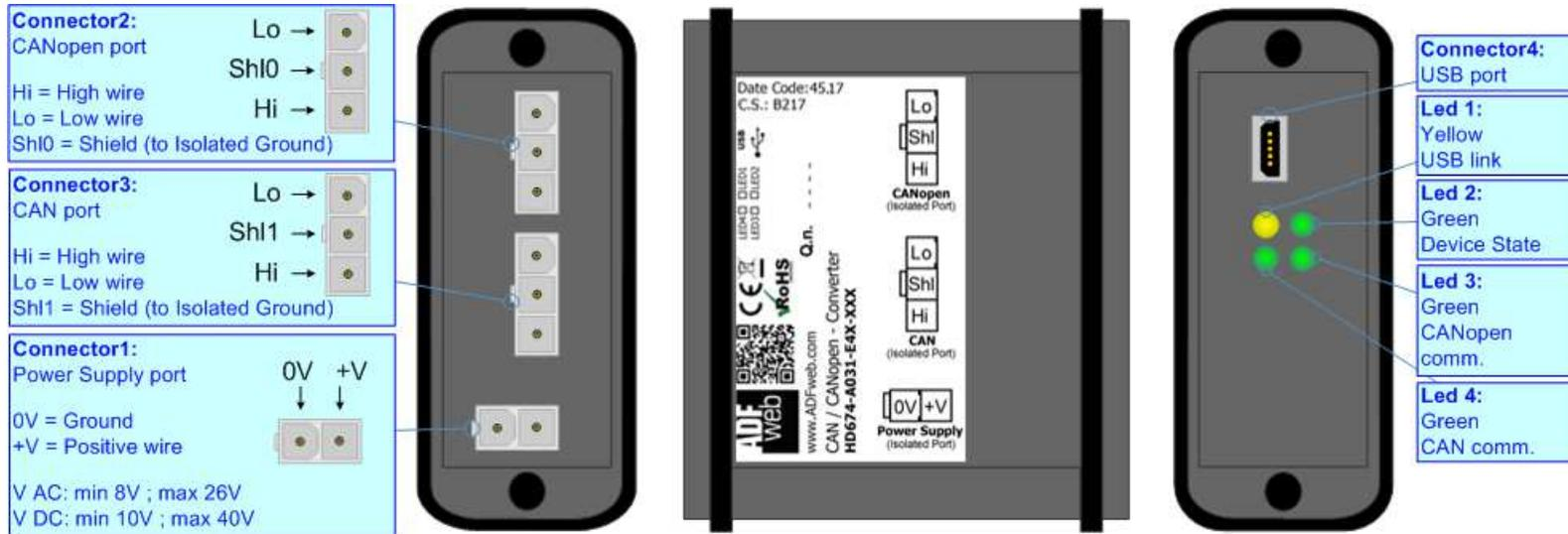
Figure 1a: Connection scheme for HD674-A031-E4x-xxx
