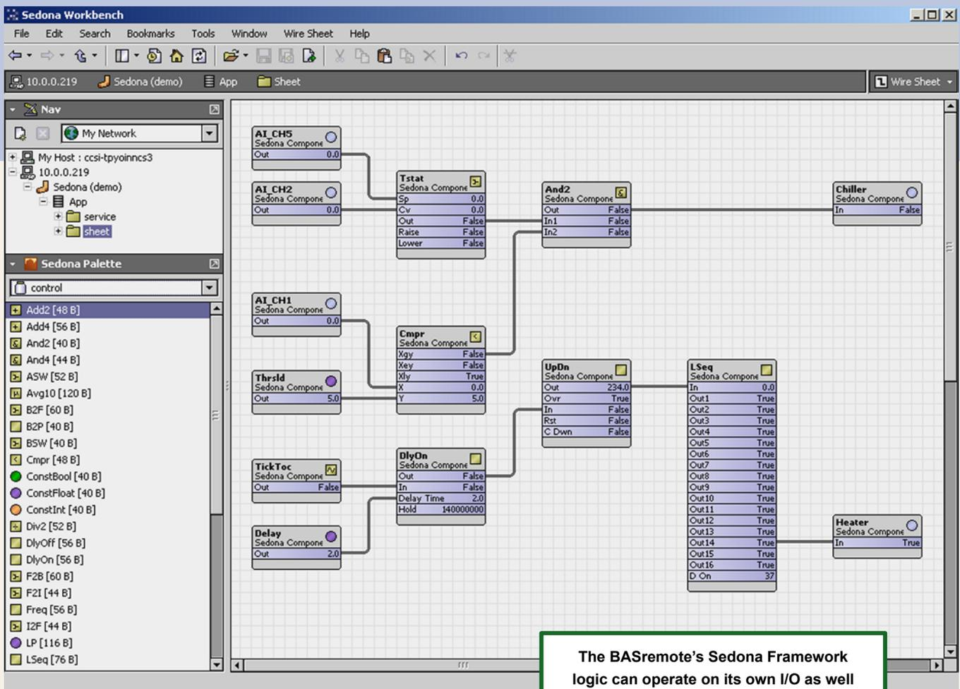
The BASremote’s Sedona Framework logic can operate on its own I/O as well as that of connected Modbus Serial or TCP devices. Also, a network connected Niagara Framework device can read or modify the operating state of the Sedona Framework function blocks.
