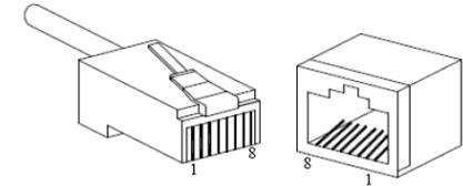
RJ 45 port support automatic MDI/MDI-X operation. That can connect the PC, Server, Converter and HUB. Pin 1, 2, 3, 4, 5, 6, 7, 8 Corresponding connections in MDI. 1→3, 2→6, 3→1, 4→7, 5→8, 6→2, 7→4, 8→5, are used as cross wiring in the MDI-X port of Converter and HUB. In MDI/MDI-X, 100/1000Base-TX PIN defines is as follows:
