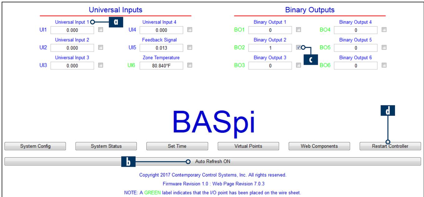
The main web page provides an overview of all real points plus access to other web pages. To configure a point, click on the point name (a) and a configuration page will appear. To observe the updated data for each point, click Auto Refresh button to ON (b). Point values can be temporarily forced by checking the box adjacent to the point (c), entering a value into the point's text
