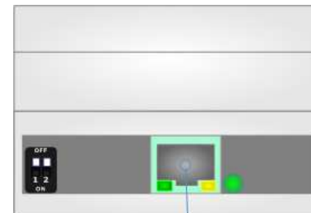
Connector3: Ethernet Port (RJ45 Plug)
