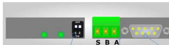
Connector5: RS232 port (D-SUB9-Male)
