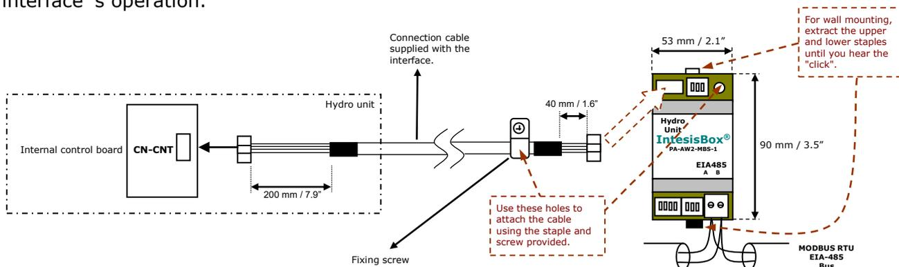
Figure 2.1 PA-AW2-MBS-1 connection diagram
