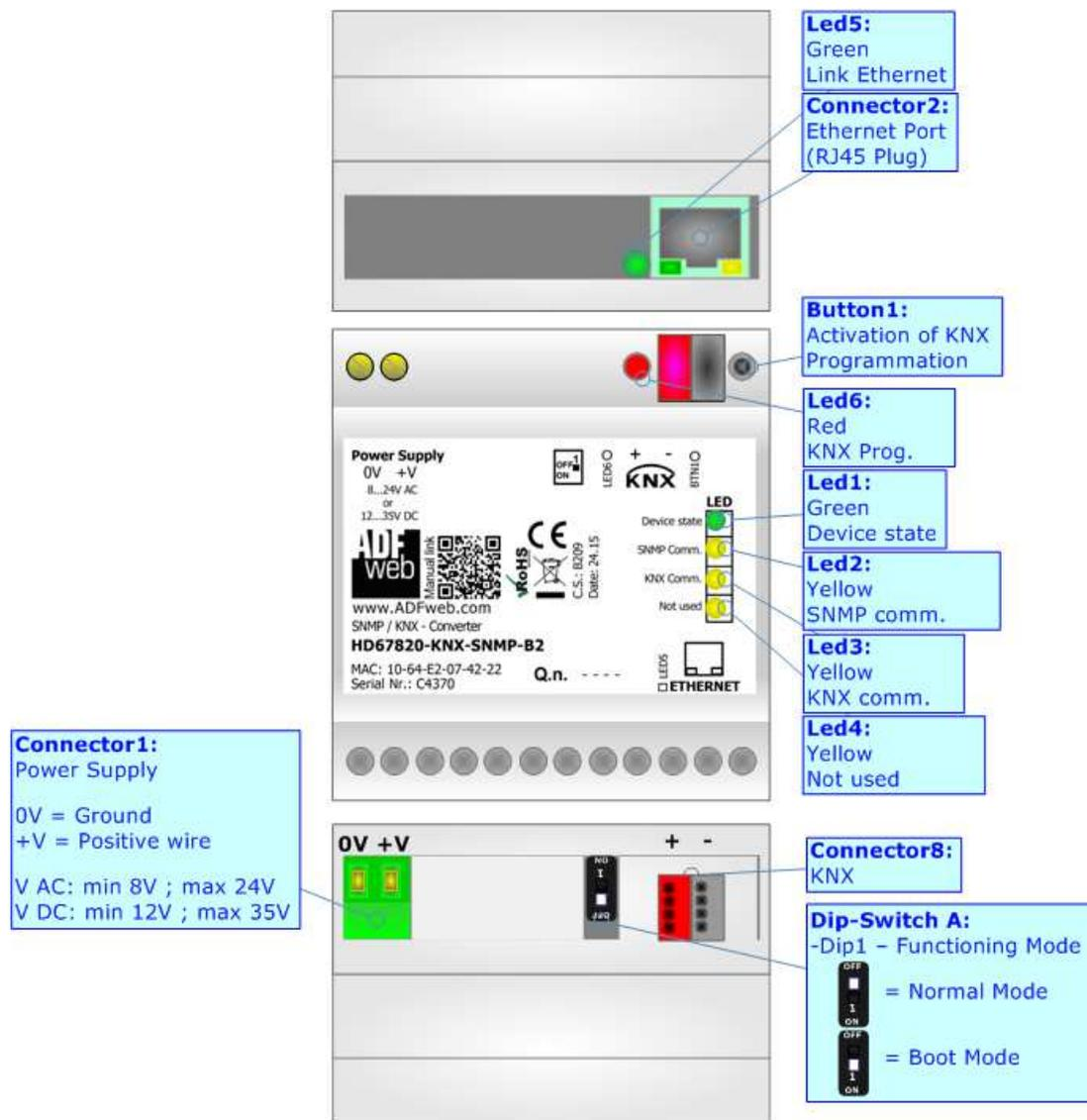
Figure 1: Connection scheme for HD67820-KNX-B2
