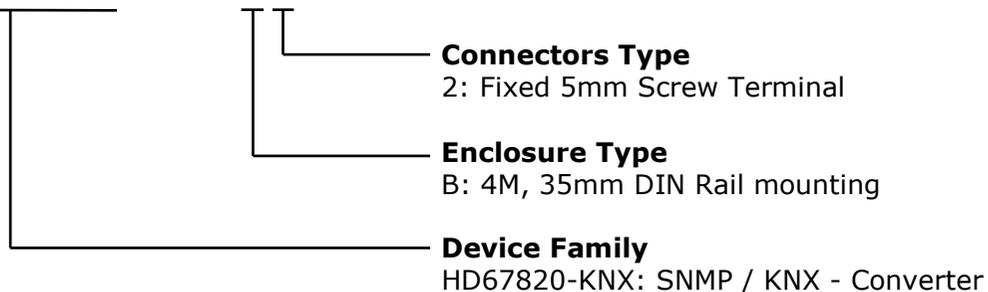
Order Code: **HD67820-KNX-B2** - SNMP / KNX – Converter
