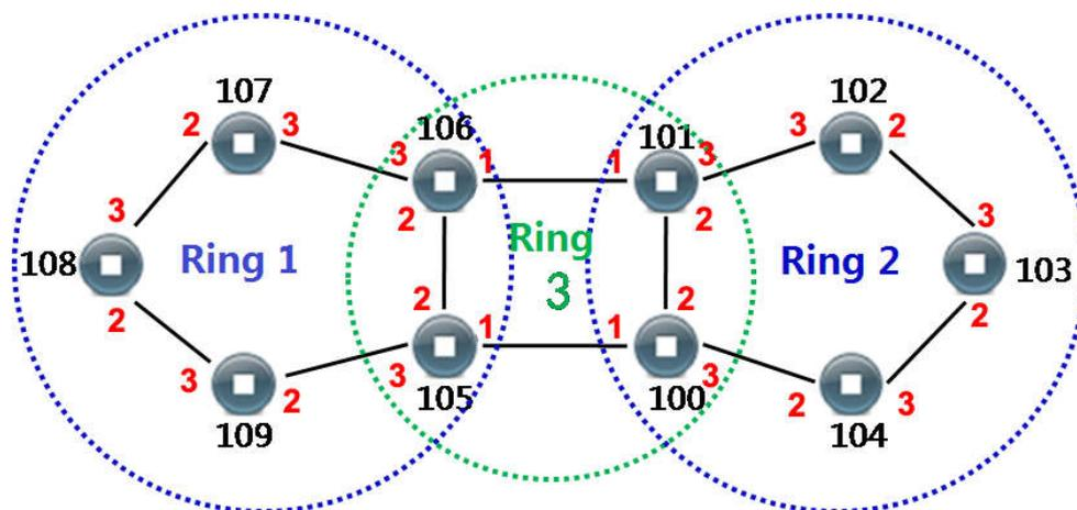
There are three rings in coupling ring. Ring 1 and Ring 2 intersect Ring 3 respectively. When setting ring in WEB interface, we can set Ring 1 and Ring 2 as single ring, Ring 3 as coupling ring. In coupling ring, we set the port in the link where the two rings intersect as control port. The Port 2 of Device 105 in the picture above is the control port. The analyses of each switch are displayed as follows:
