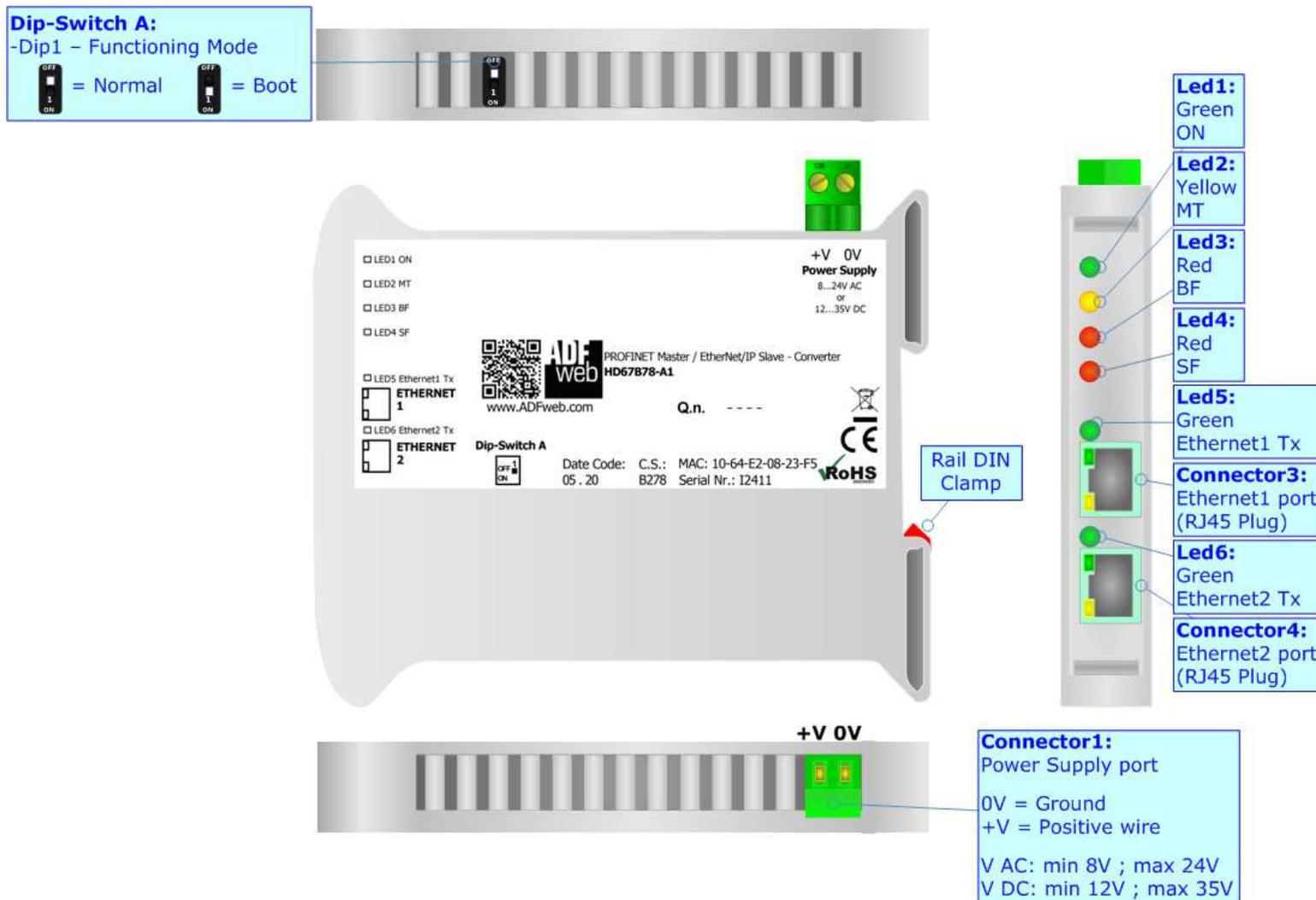
Figure 1: Connection scheme for HD67B78-A1
