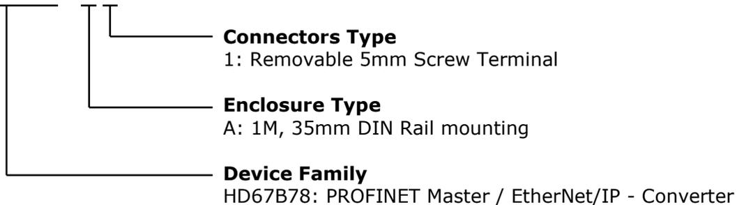
Order Code: **HD67B78-A1** - PROFINET Master / EtherNet/IP - Converter
