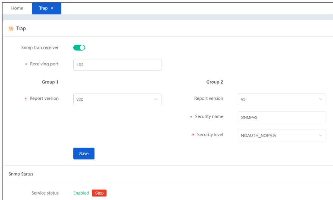
The main element configuration description of Trap settings interface:
