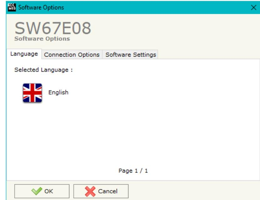
In the section “Connection Options”, it is possible to check if there are some updatings of the software compositor in ADFweb.com website. Checking the option “**Check Software Update at Start of Program**”, the SW67E08 checks automatically if there are updatings when it is launched.
