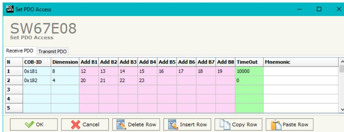
Figure 7a: "Set PDO Access – Receive PDO" window
