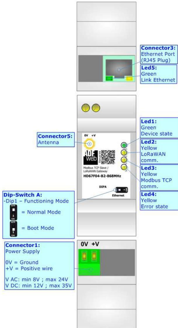
Figure 1: Connection scheme for HD67F04-B2-xxxMHz
