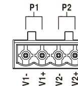
Model XIII, XIV devices of this series support dual DC power input, and provide 4-pin terminals with a spacing of 5.08 mm. The power supply supports power redundancy and has anti-reverse connection function. Power supply range: 12~48VDC. The pins of power supply terminal are shown in the left figure.
