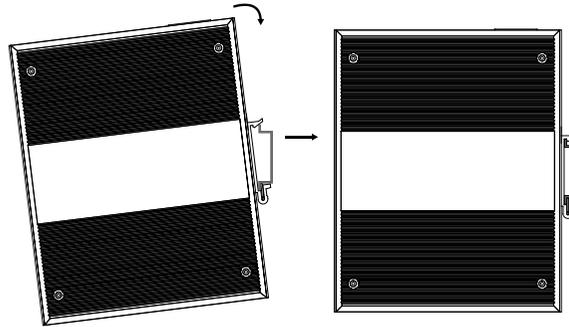
Step 1 Check if the DIN-Rail mounting kit is installed firmly.
