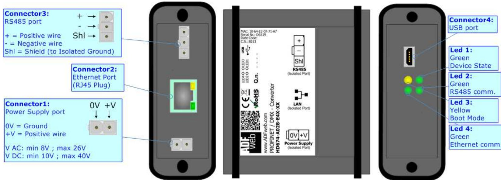
Figure 1a: Connection scheme for HD674-A028-E4x-xx
