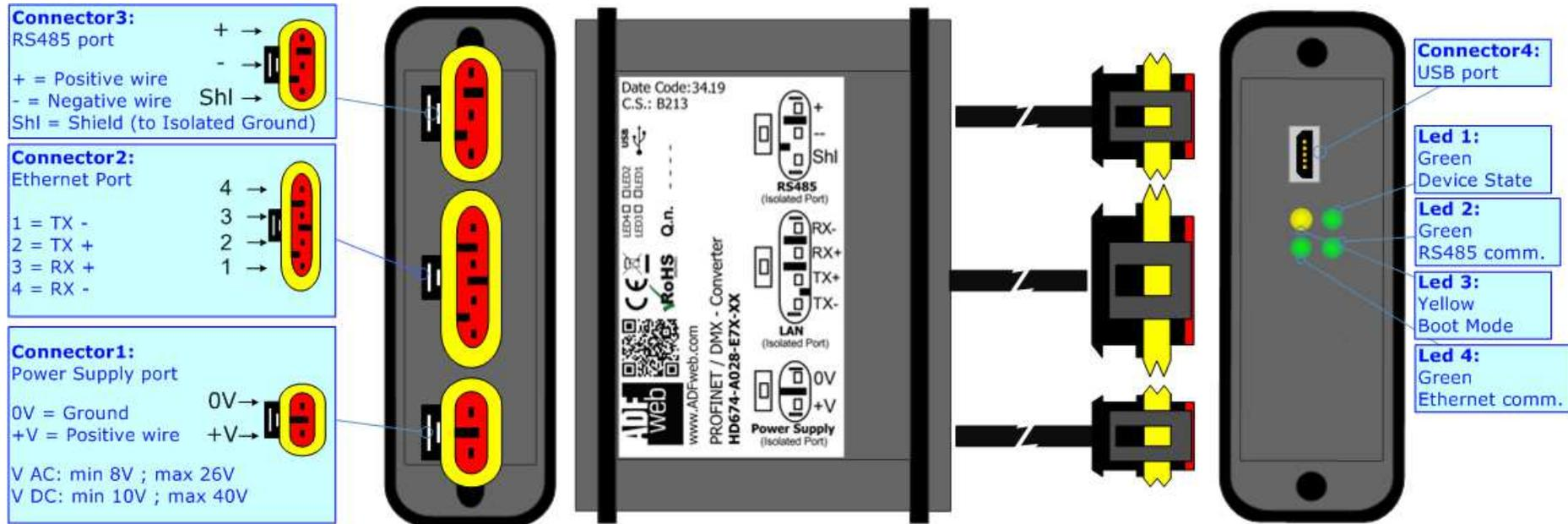
Figure 1b: Connection scheme for HD674-A028-E7x-xx
