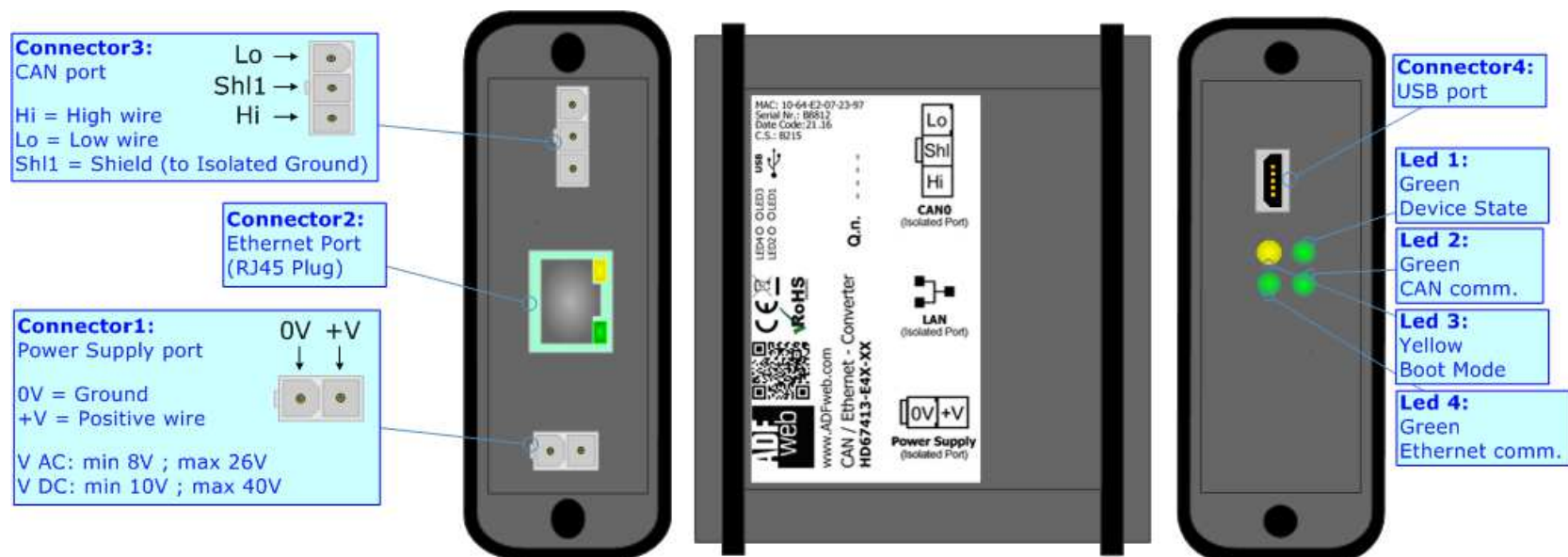
Figure 1a: Connection scheme for HD67413-E4x-xx
