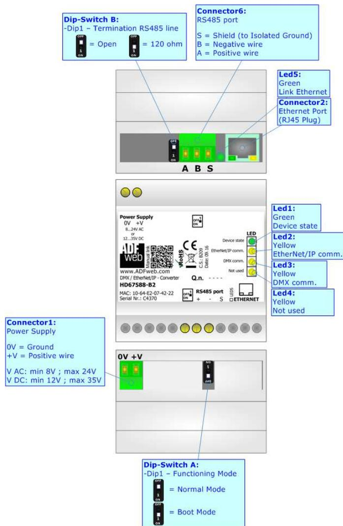
Figure 1: Connection scheme for HD67588-B2
